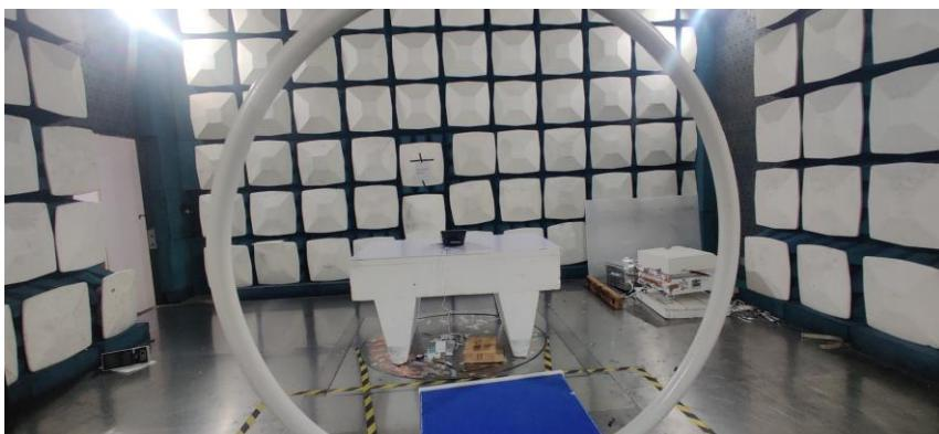
**Radiated spurious emissions (30MHz-1GHz)**
