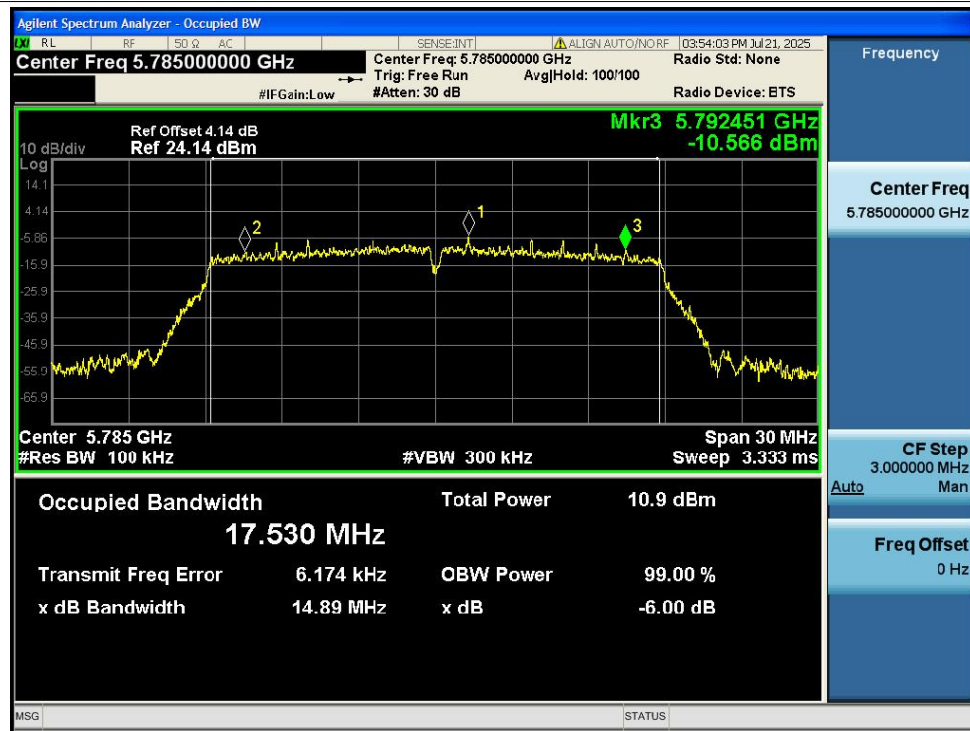
-6dB Bandwidth NVNT n20 5825MHz Ant2
