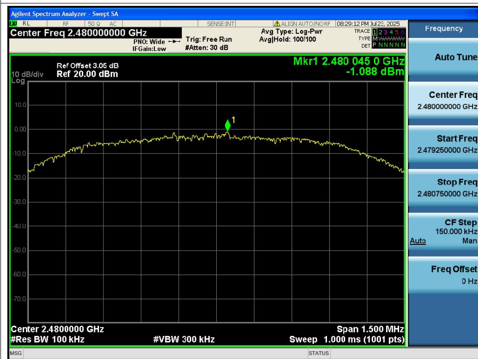
Tx. Spurious NVNT 2-DH5 2480MHz Ant1 Emission
