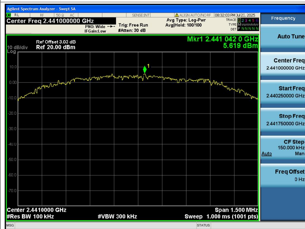
Tx. Spurious NVNT 3-DH5 2441MHz Ant1 Emission
