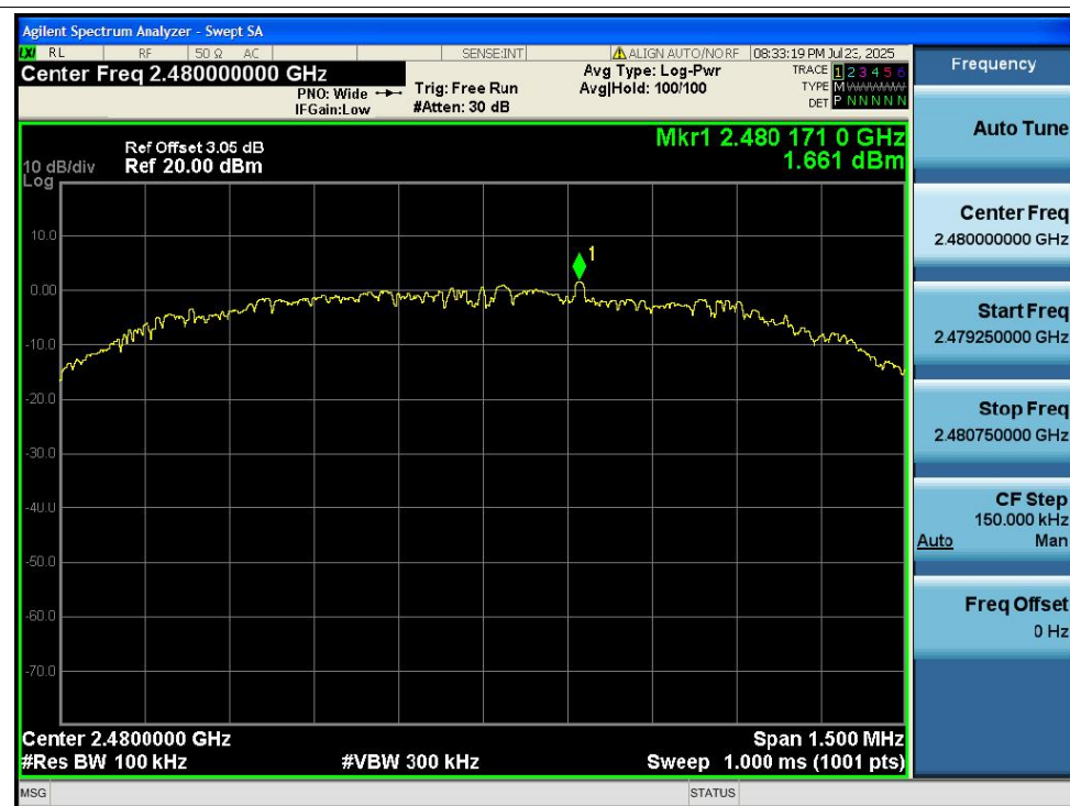
Tx. Spurious NVNT 3-DH5 2480MHz Ant1 Emission
