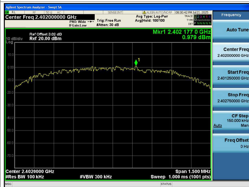
Tx. Spurious NVNT 3-DH5 2402MHz Ant1 Emission
