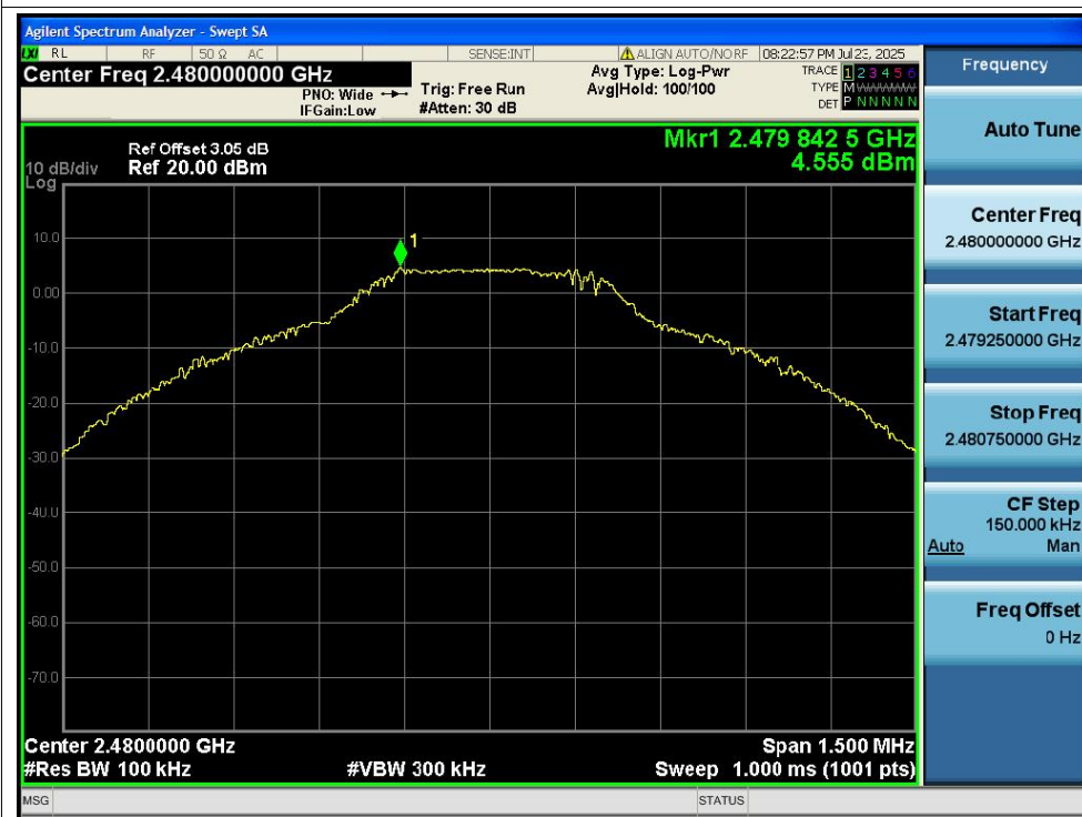
Tx. Spurious NVNT 1-DH5 2480MHz Ant1 Emission
