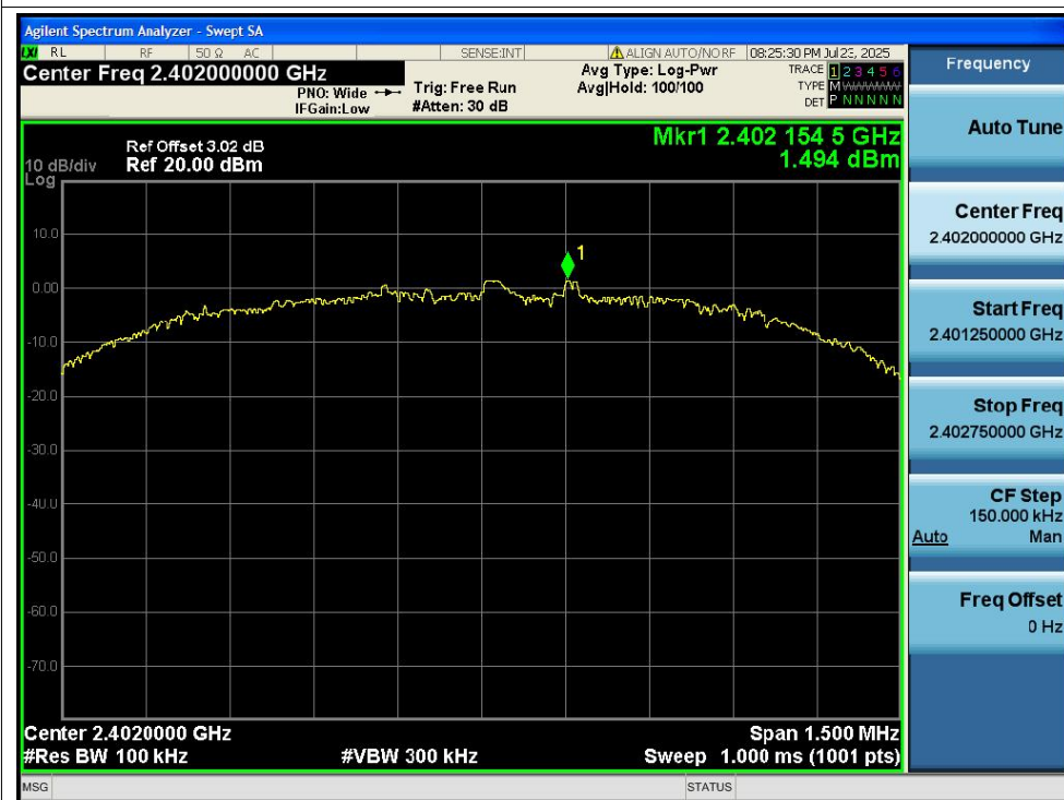
Tx. Spurious NVNT 2-DH5 2402MHz Ant1 Emission
