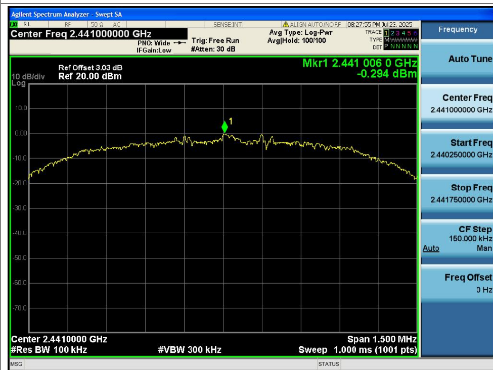
Tx. Spurious NVNT 2-DH5 2441MHz Ant1 Emission
