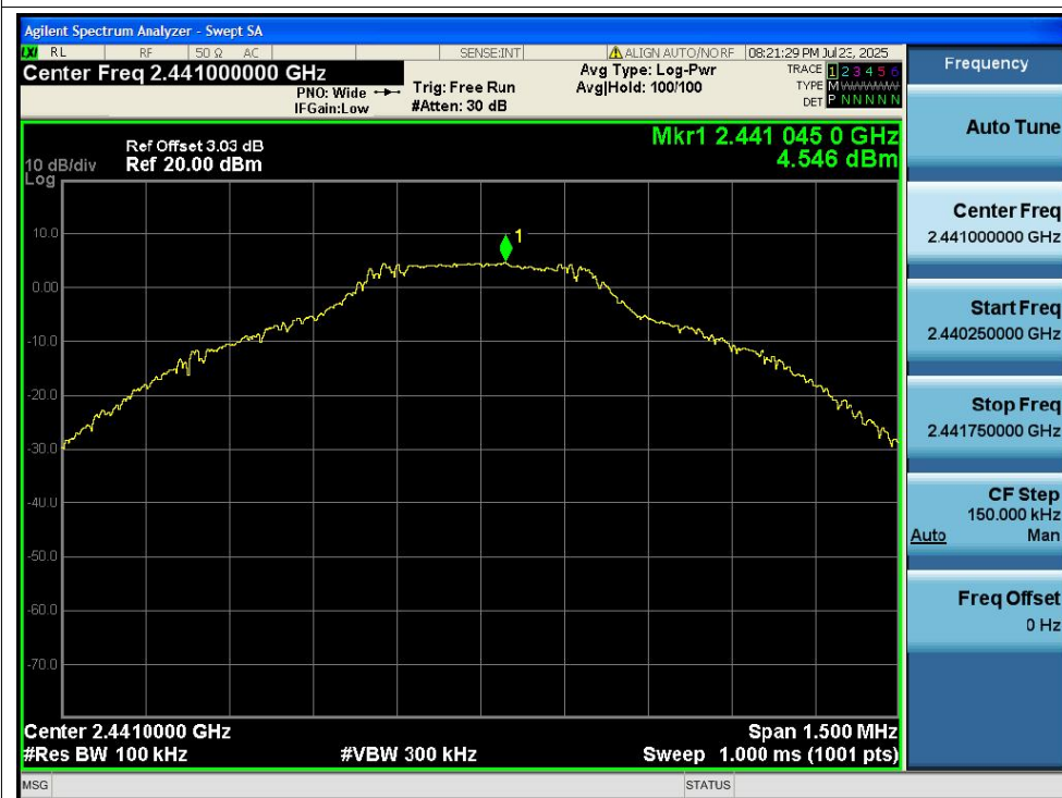
Tx. Spurious NVNT 1-DH5 2441MHz Ant1 Emission
