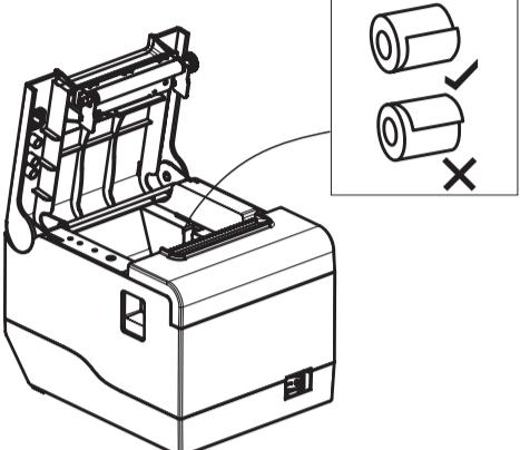
Remove the used roll paper core if any, and insert the roll paper. The correct direction of the paper is shown in the illustration below.
