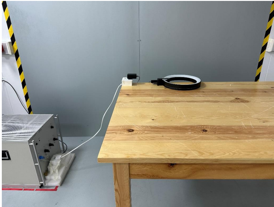
Radiated Emission Test Setup Photo - Below 1GHz
