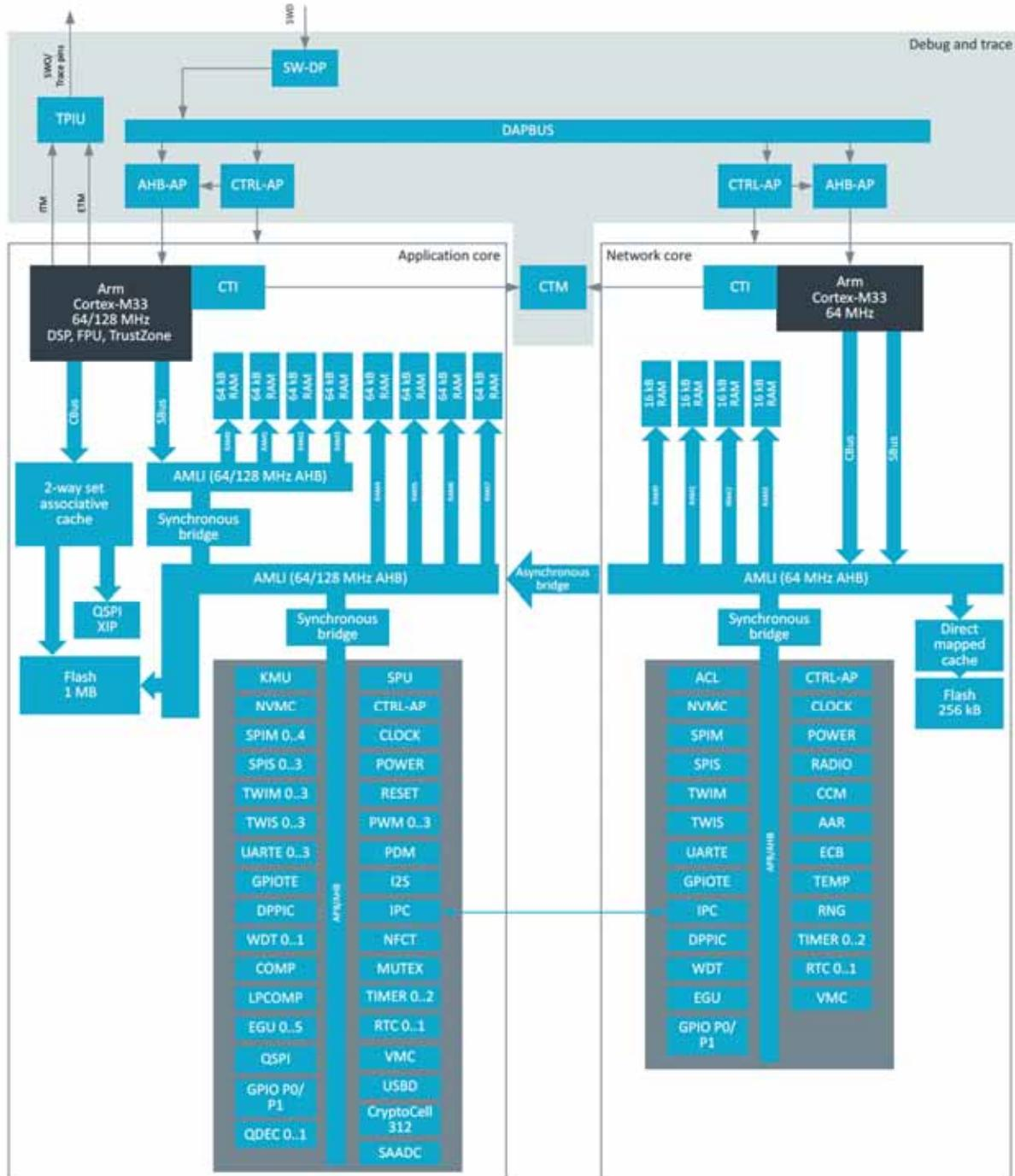
nRF5340 is a wireless ultra-low power multiple core System on Chip (SoC) integrating two fully programmable Arm Cortex M33 processors, advanced security features, a range of peripherals, and a multi protocol 2.4 GHz transceiver. transceiver supports Bluetooth low energy.
