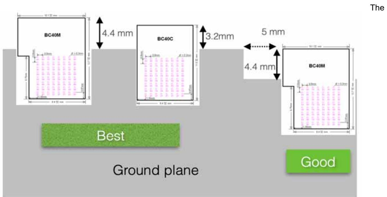
The following figure shows recommended mounting of BC40C module on the host PCB.
