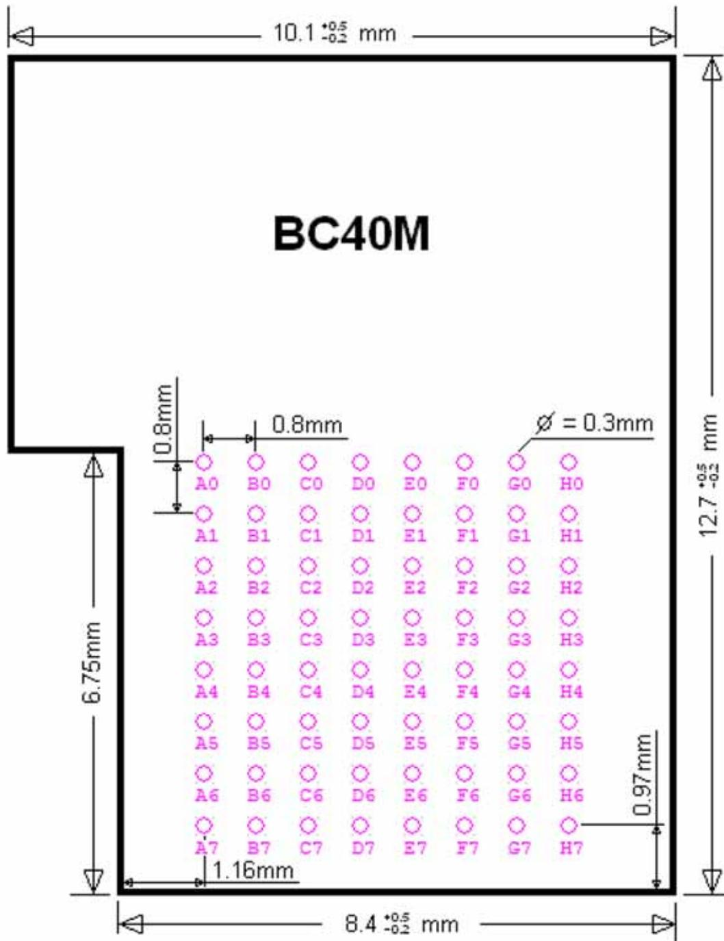
mechanical drawings, top view. Module size is 8.4 (10.1) x 12.7 x 1.5mm, L-shape.
