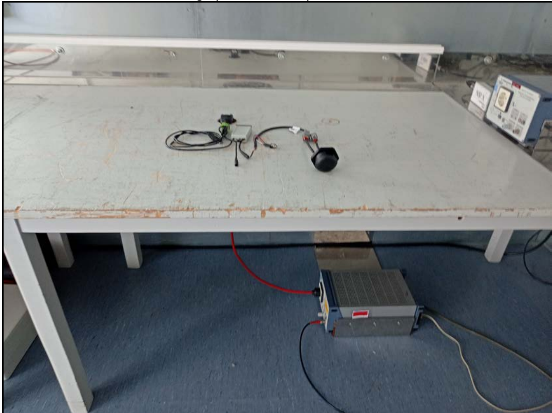
Photo 1: Photograph of Test setup 1 conducted emission
