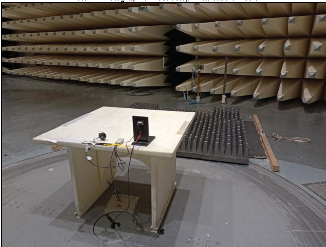
Photo 4: Photograph of Test setup 1 radiated emission
