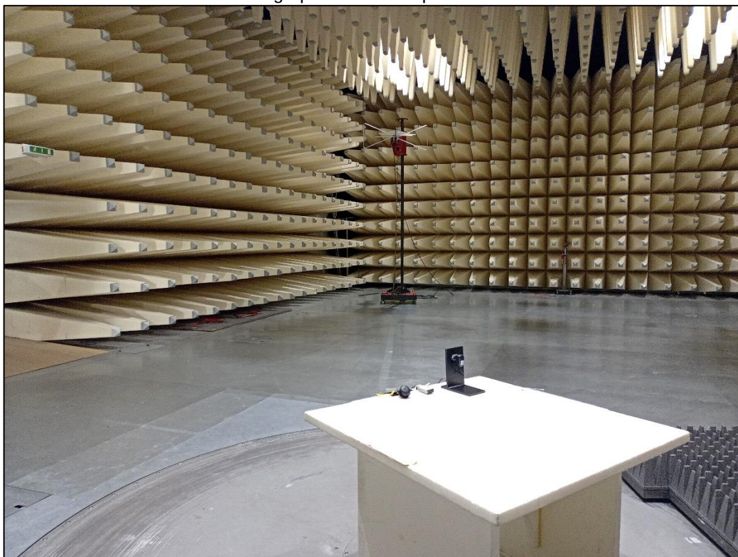
Photo 5: Photograph of Test setup 2 radiated emission
