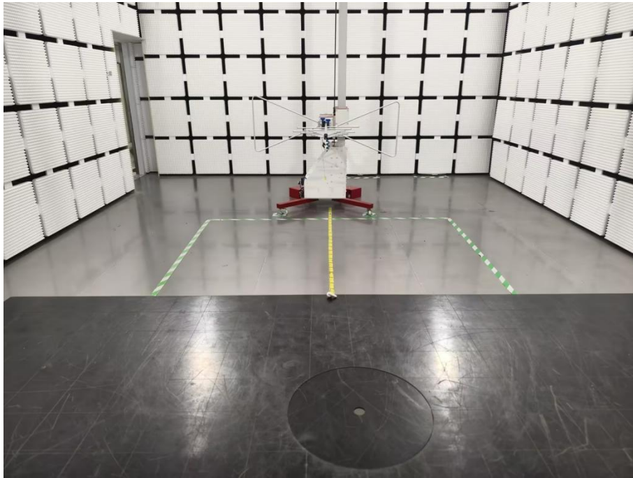
Spurious Radiation Emissions Test (<1G)
