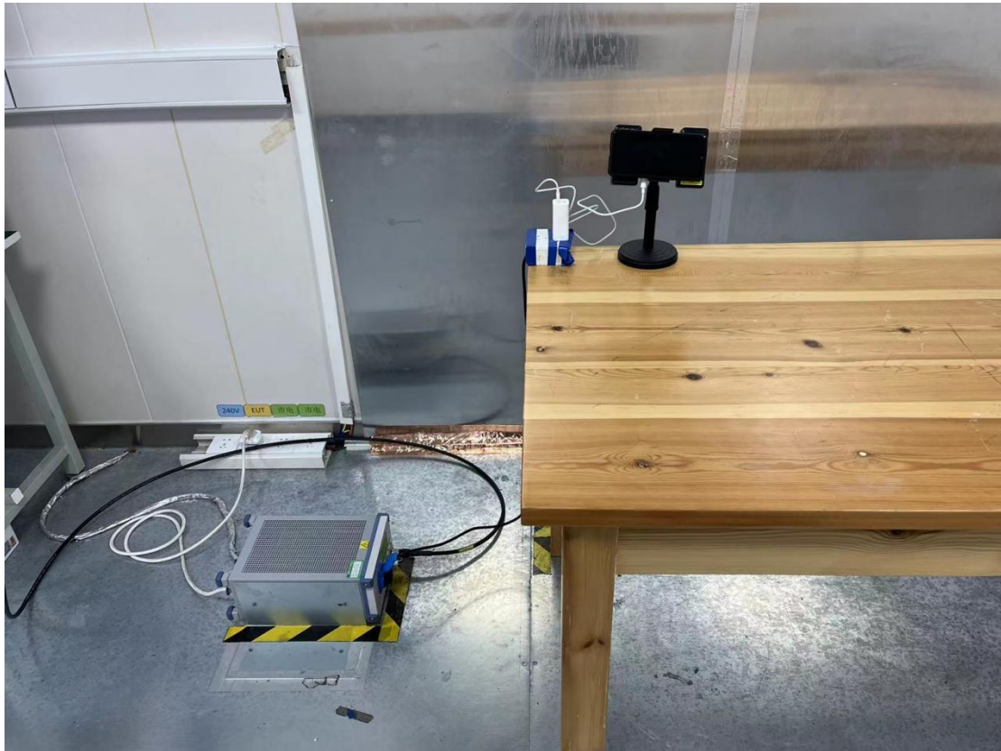
Conducted emission test setup
