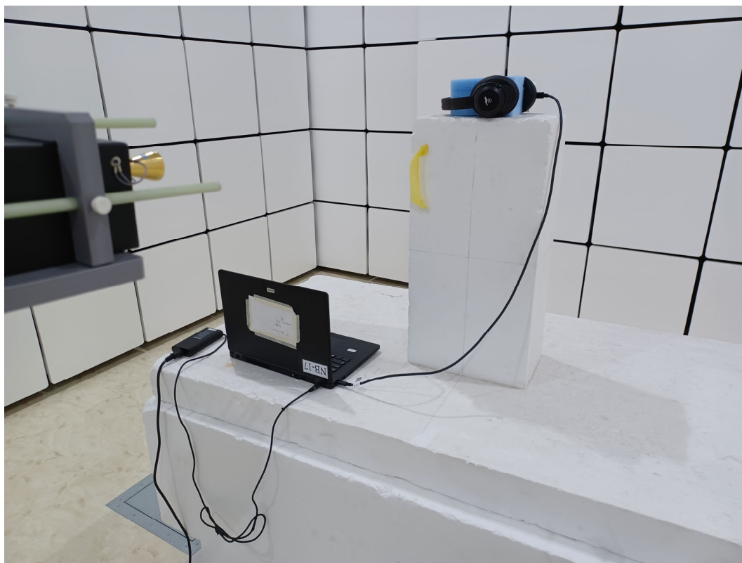
Back View of Radiated Test (Horn)
