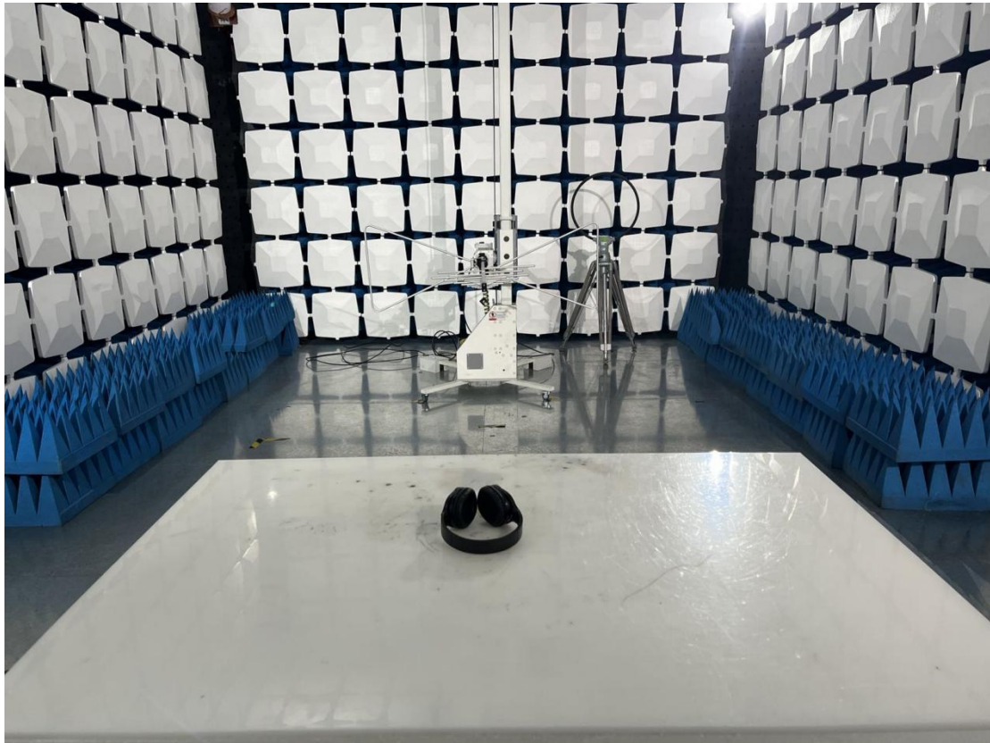
Blow 1GHz for radiated emission test setup
