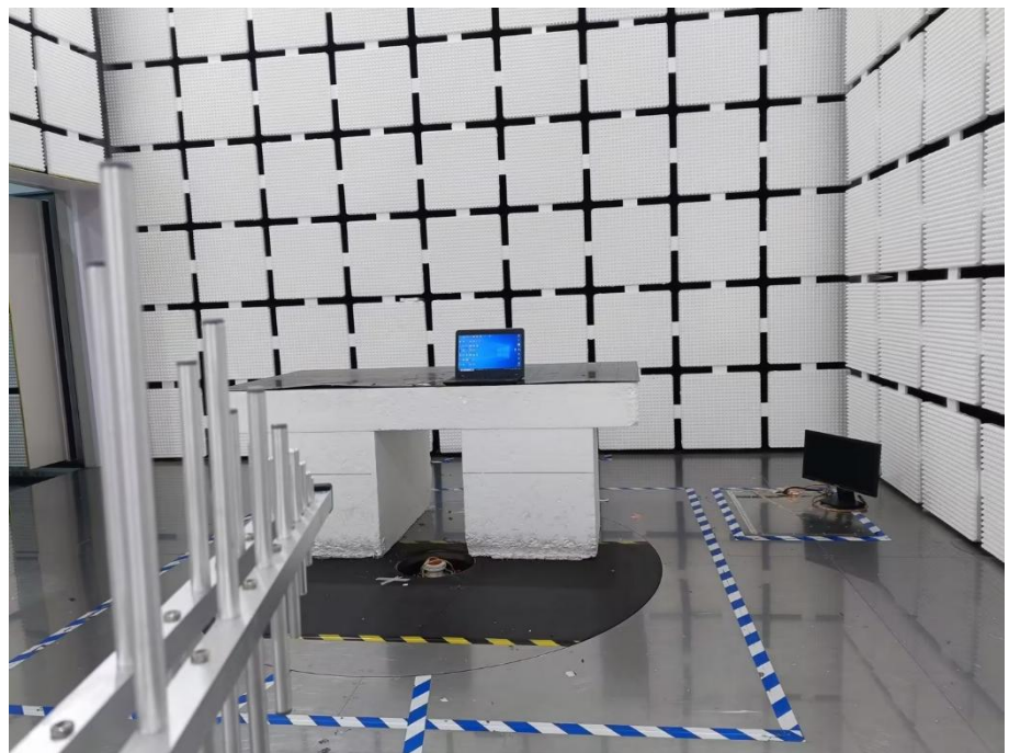
Radiation Emission Test Setup (30MHz to 1GHz)
