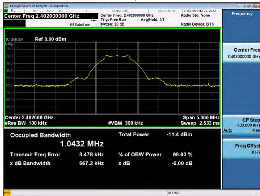
6 dB Bandwidth plot (Low-CH 0)
