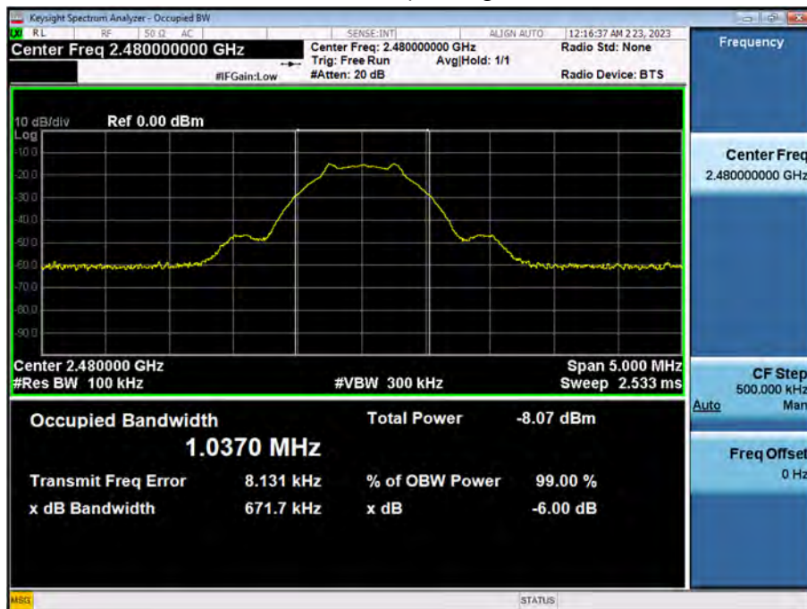
6 dB Bandwidth plot (High-CH 39)
