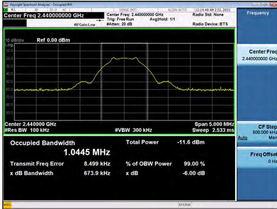
6 dB Bandwidth plot (Mid-CH 19)
