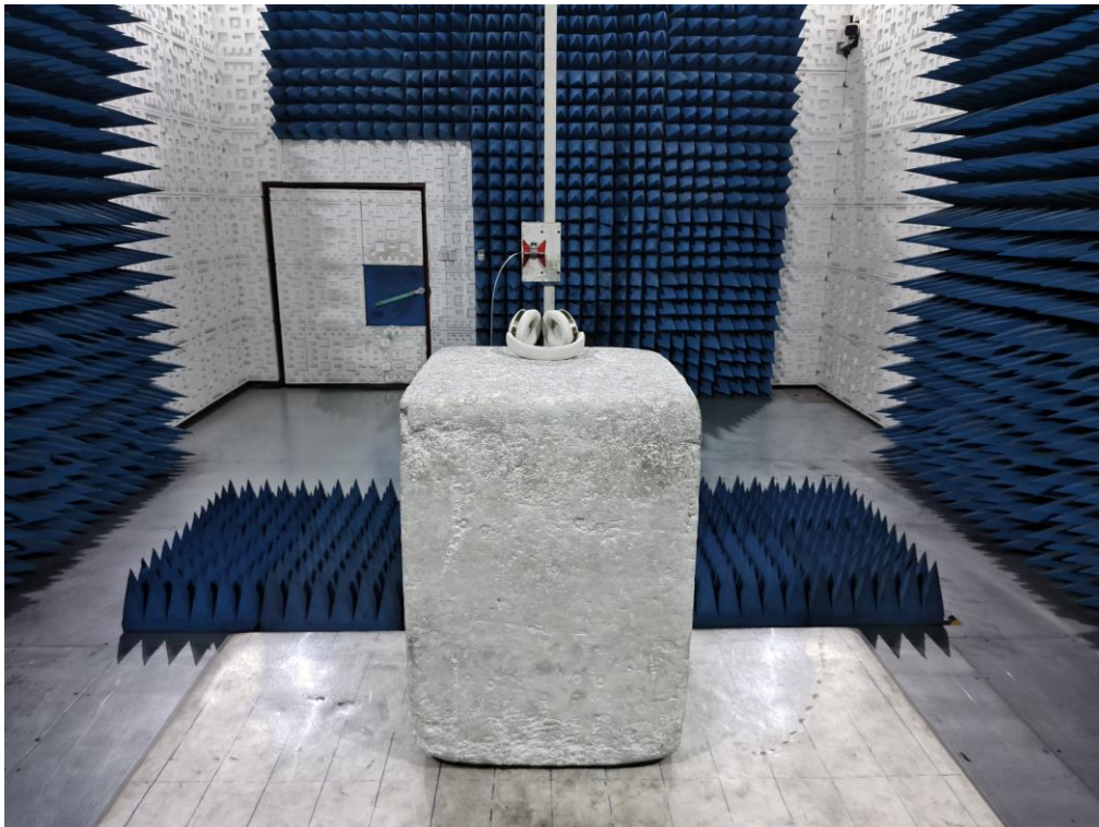
RADIATED EMISSION TEST SETUP ABOVE 1GHz
