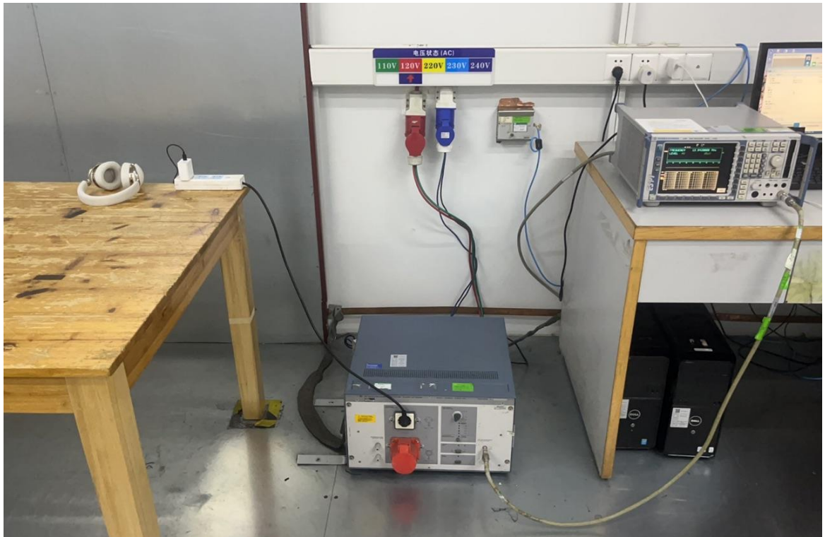
AC POWER LINE CONDUCTED TEST SETUP
