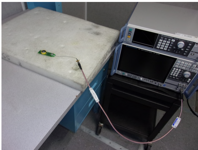
Photo 1.2-1 – Conducted Test Setup
