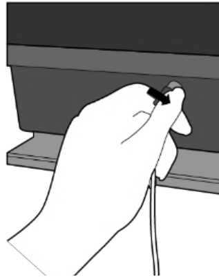
Step 2: Twist the other end of the Handpiece Tubing onto the front of the Monitor Enclosure.
