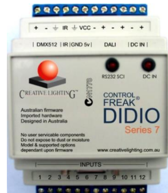
Optional DIDIO® – a convenient din mount combination of integral modules of DALI power supply 22Vdc 245mA, SCI Serial Communications Interface, and DALI Scene Controller with up to 12 i/o lines for switches and sensors eg manual DALI line emergency override, momentary push buttons, dry contacts from sensors. Up to 4 of the 12 i/o lines can be opto-isolated outputs eg as 24vdc outputs to drive 24v coils of contactors
