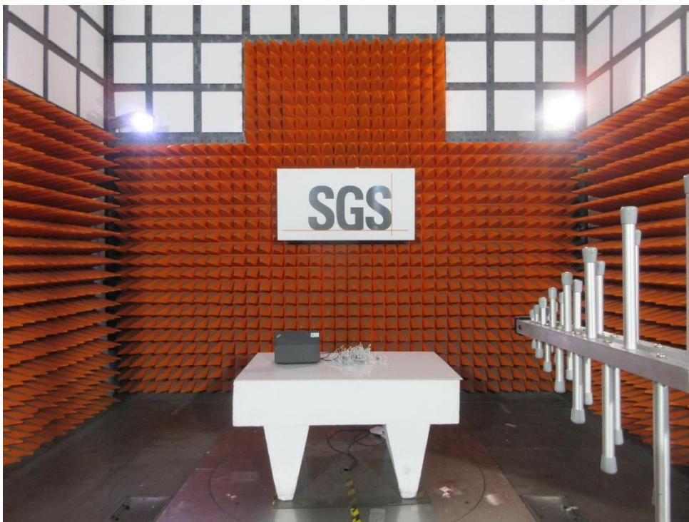
**Radiated Spurious Emissions Above 1GHz**
