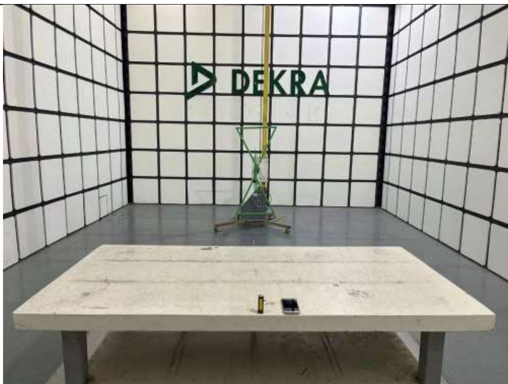
Description: Rear View of Radiated Disturbance Test Setup (Below 1 GHz)
