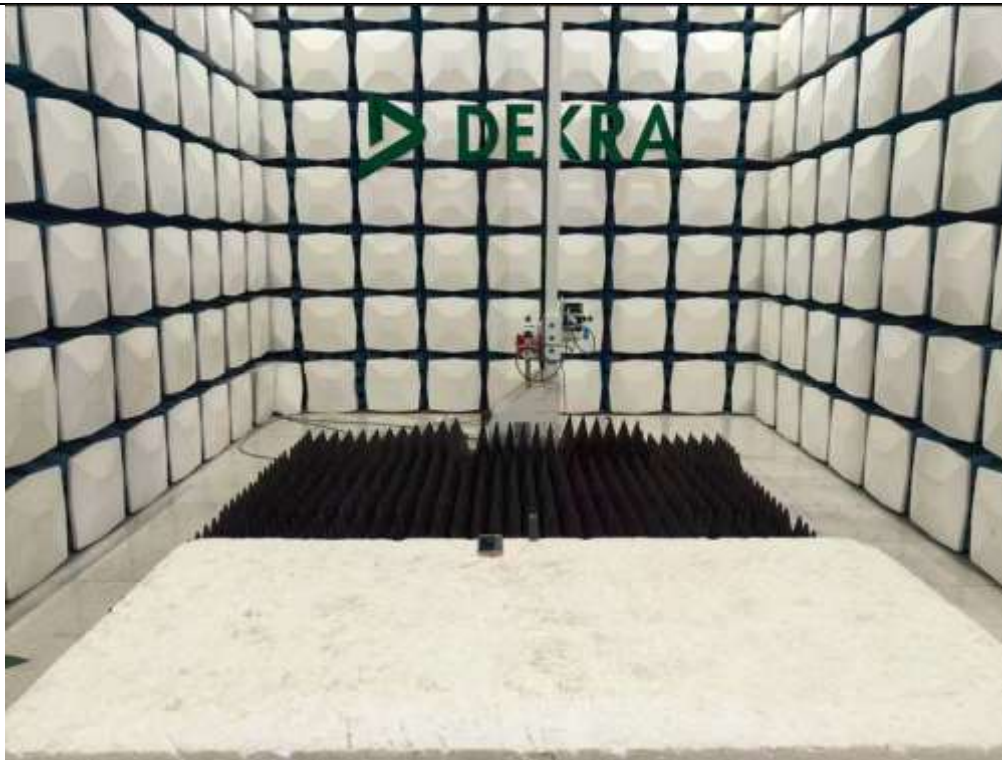
Description: Rear View of Radiated Disturbance Test Setup (Above 1 GHz)
