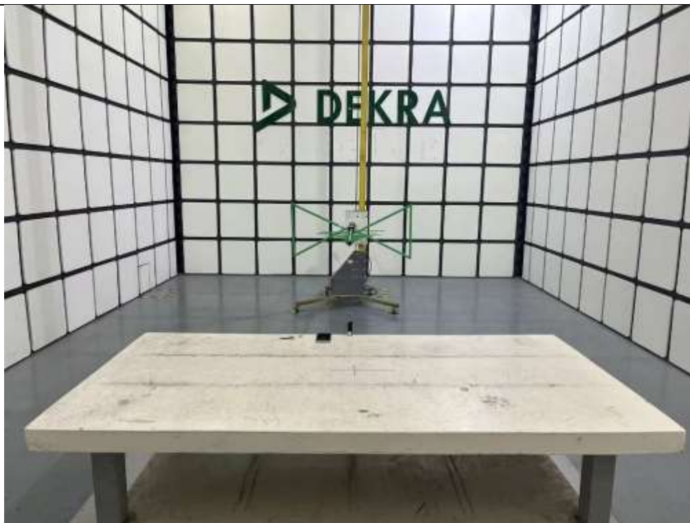
Description: Rear View of Radiated Disturbance Test Setup (Below 1 GHz)
