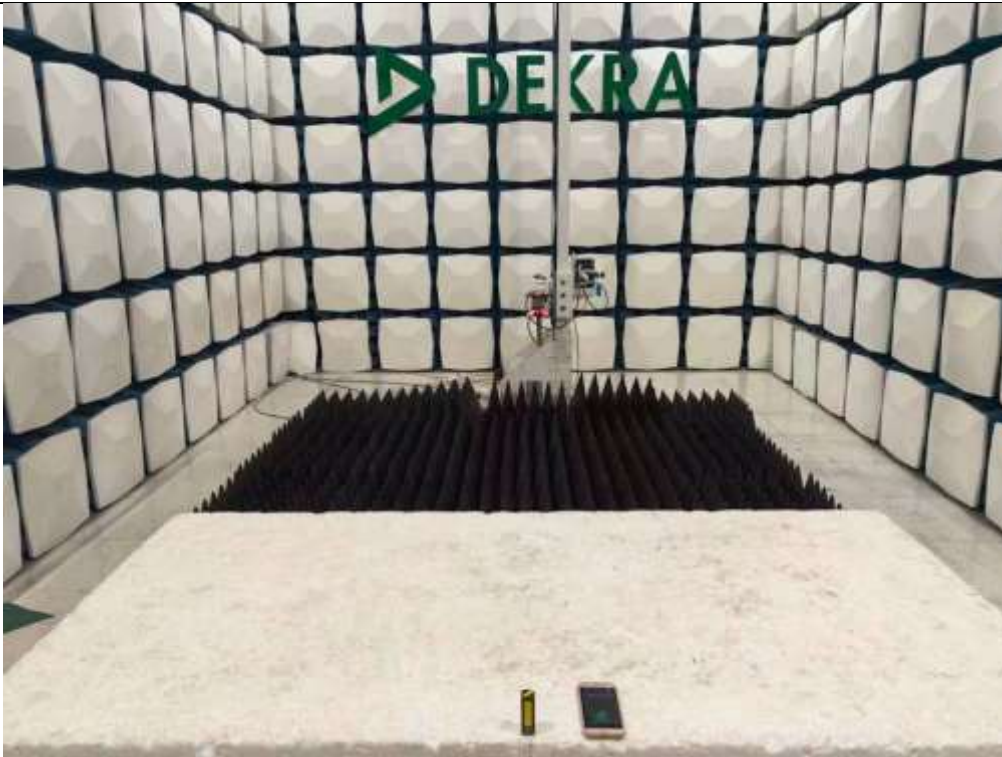
Description: Rear View of Radiated Disturbance Test Setup (Above 1 GHz)
