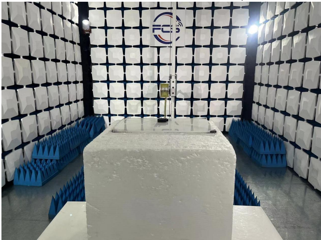
Above 1GHz for radiated emission test setup
