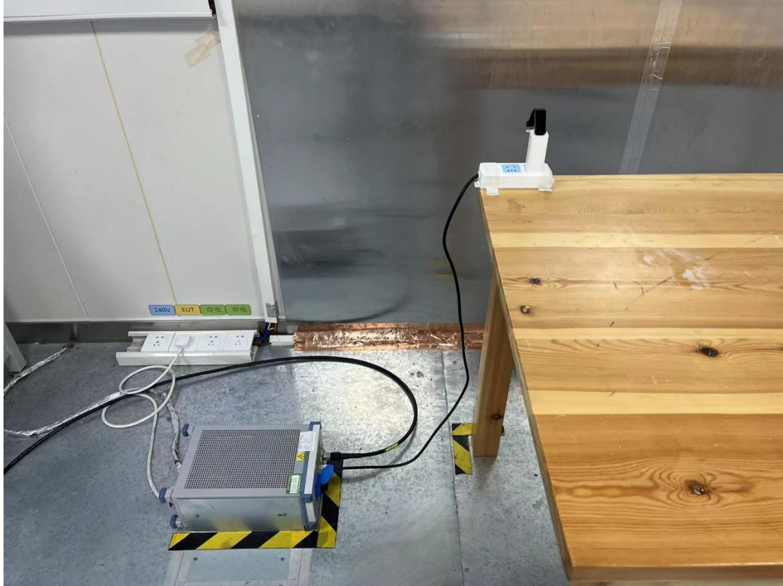
Conducted emission test setup
