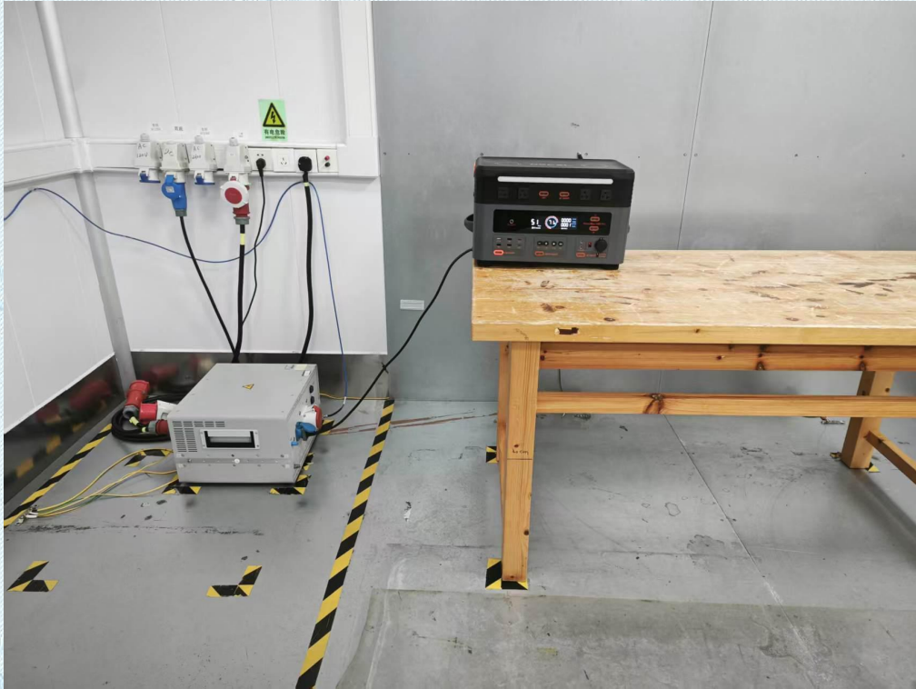
Conducted Emission at AC power line
