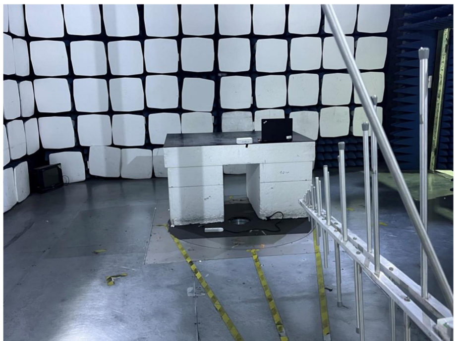
Radiation Emission Test Setup (30MHz to 1GHz)
