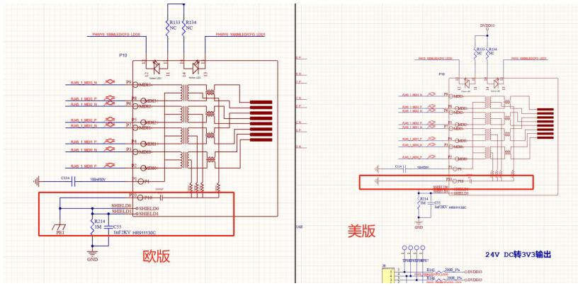
2. The capacitance values of C135 and C136 are changed from 20pf to 27pf
