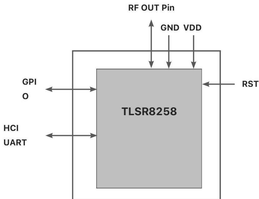
Picture 1-3 Function Block Diagram
