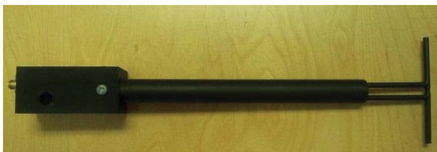
Figure 1 – MVG COMOSAR Validation Dipole
