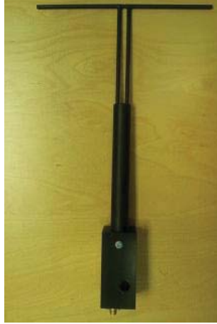
Figure 1 – MVG COMOSAR Validation Dipole
