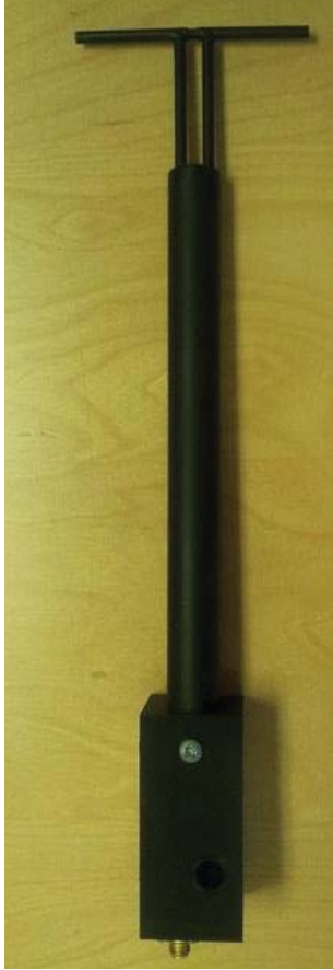
Figure 1 – MVG COMOSAR Validation Dipole
