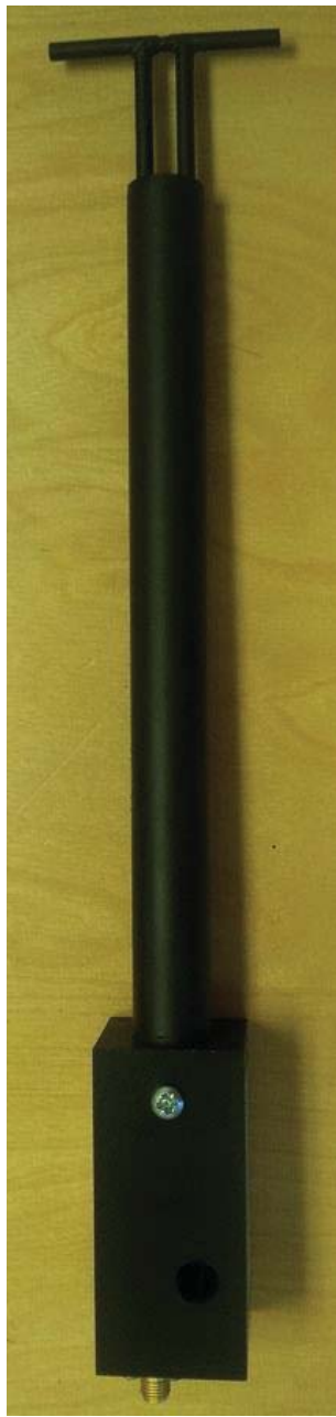
Figure 1 – MVG COMOSAR Validation Dipole
