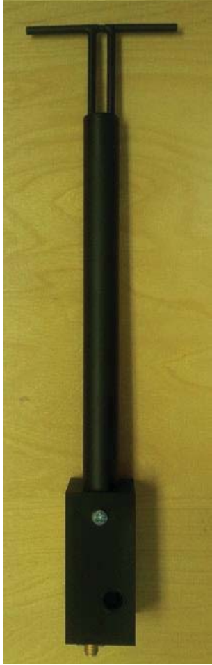
Figure 1 – MVG COMOSAR Validation Dipole
