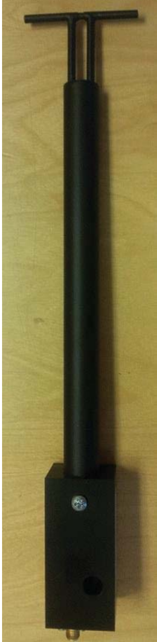
Figure 1 – MVG COMOSAR Validation Dipole
