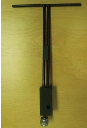
Figure 1 – MVG COMOSAR Validation Dipole
