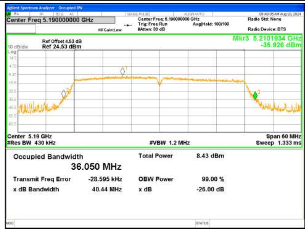
-26dB Bandwidth NVNT n40 5190MHz Ant2
