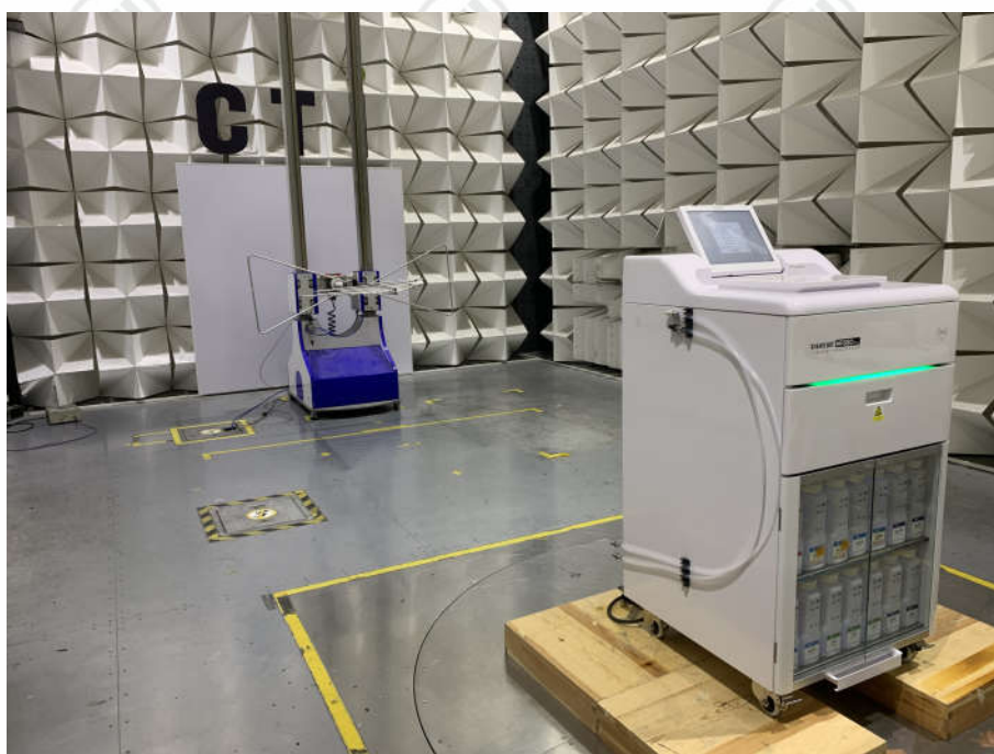
Radiated Spurious Emissions Test Setup (30MHz~1GHz)
