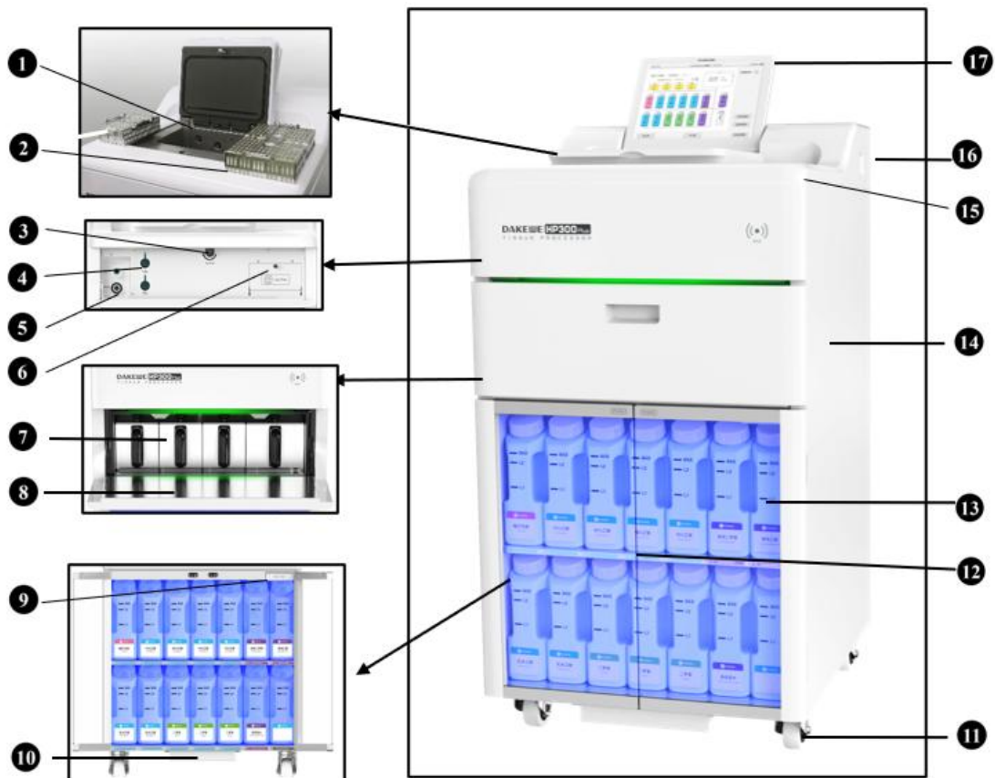
Figure 2 Front of HP300 Plus Automatic Tissue Processor
