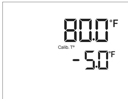
1. Long press the **Setting Button** for 5 seconds, and the Temperature Calibration page will be displayed.
