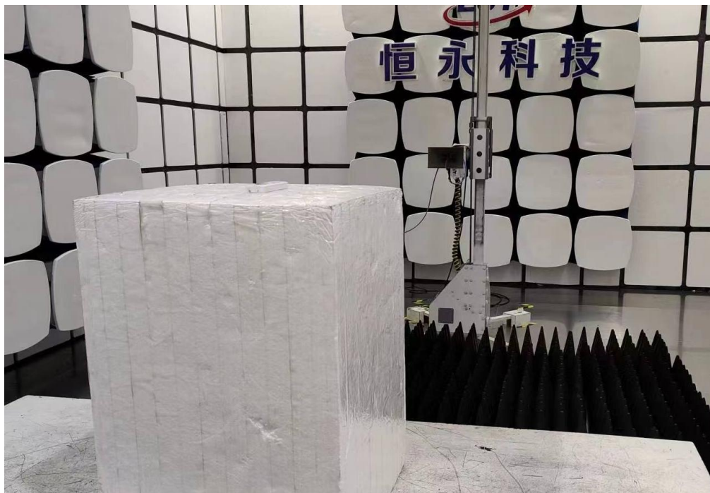
Radiated emission test: Above 1GHz
