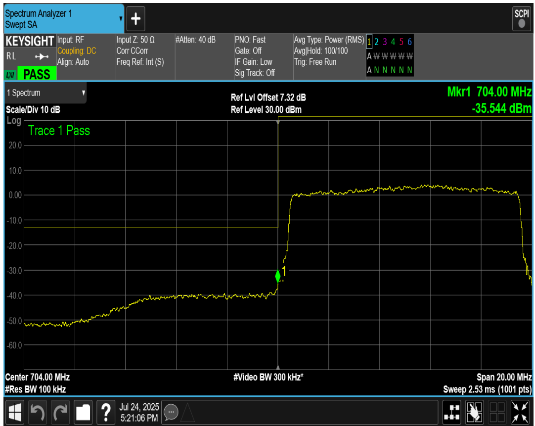
Band17 QAM16 BW=10MHz Channel=23800 RB Size=50 Position=#0
