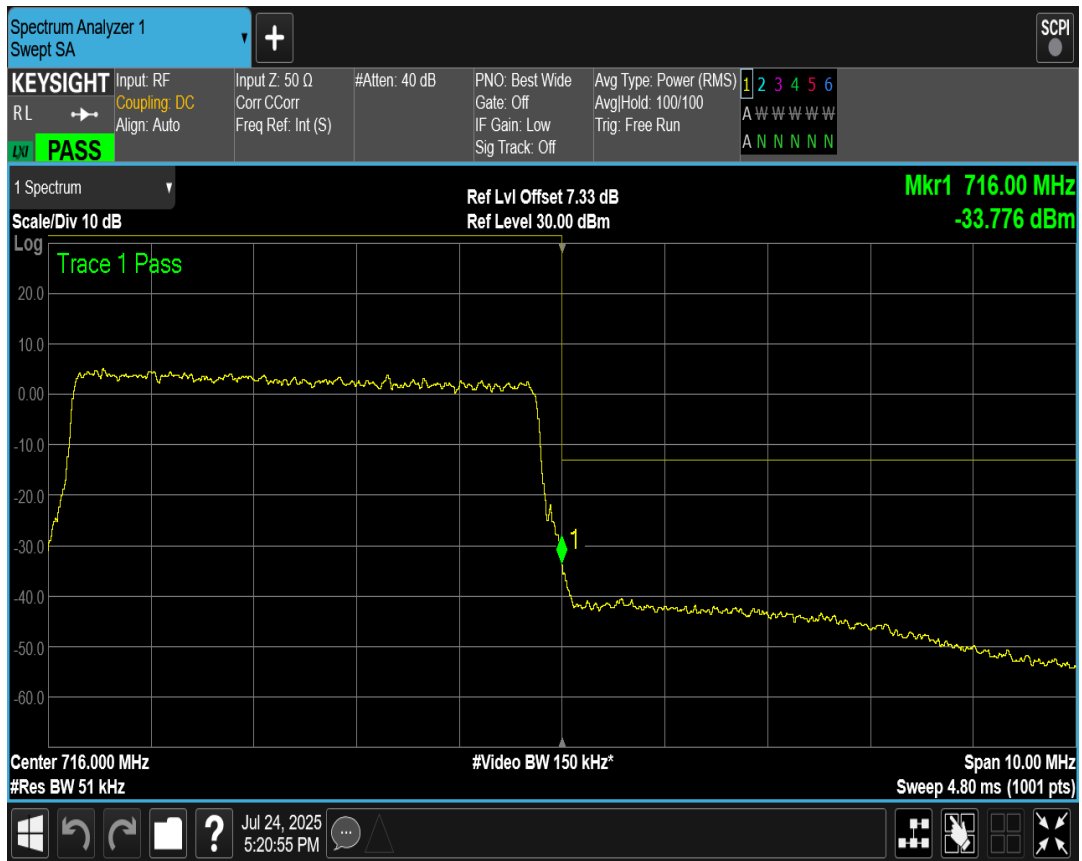
Band17 QPSK BW=5MHz Channel=23755 RB Size=25 Position=#0
