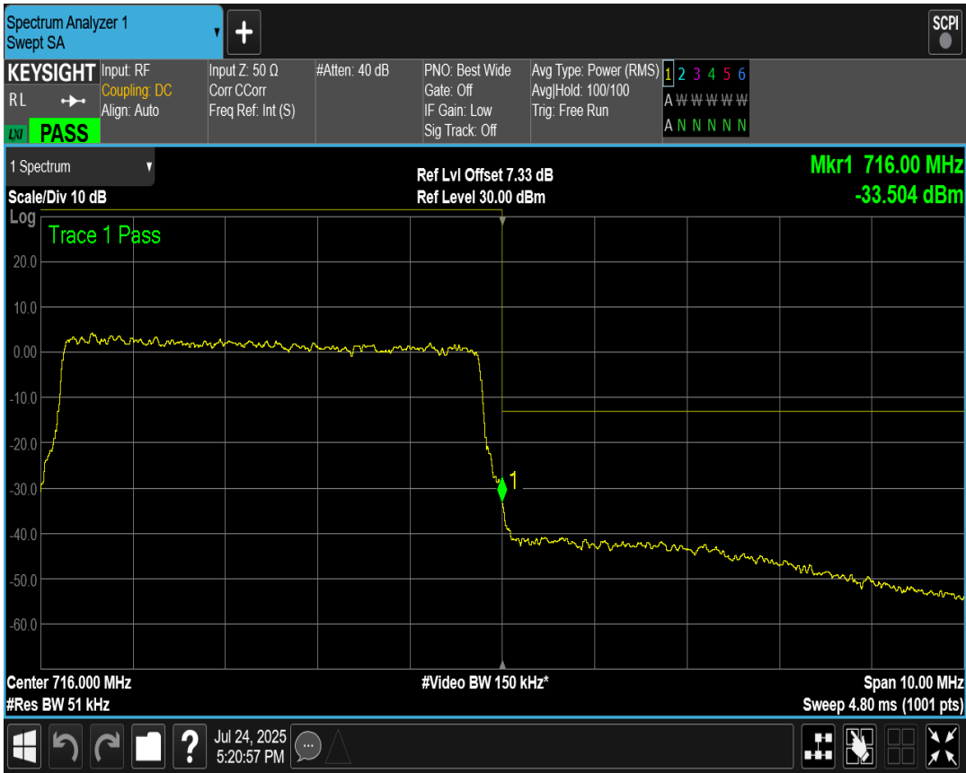
Band17 QPSK BW=10MHz Channel=23780 RB Size=50 Position=#0
