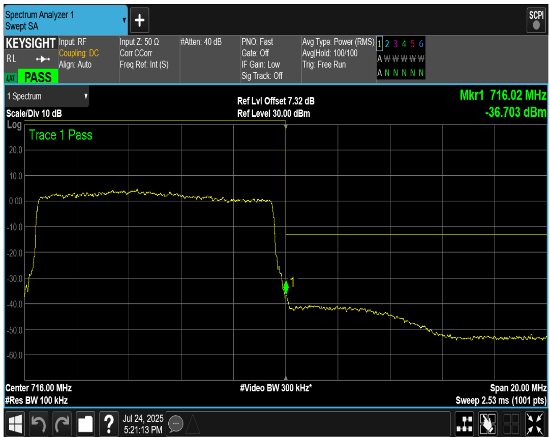
Band17 QPSK BW=5MHz Channel=23825 RB Size=25 Position=#0
