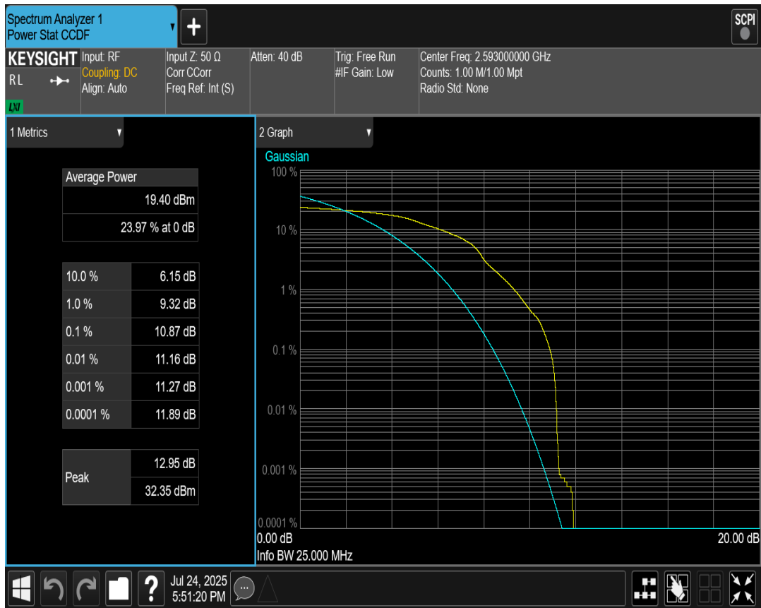
Band41 QAM16 BW=5MHz Channel=40620 RB Size=1 Position=#0
