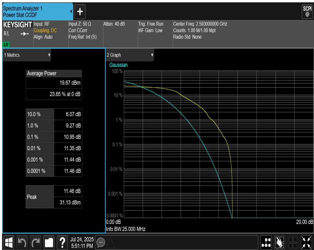
Band41 QPSK BW=20MHz Channel=40620 RB Size=1 Position=#0
