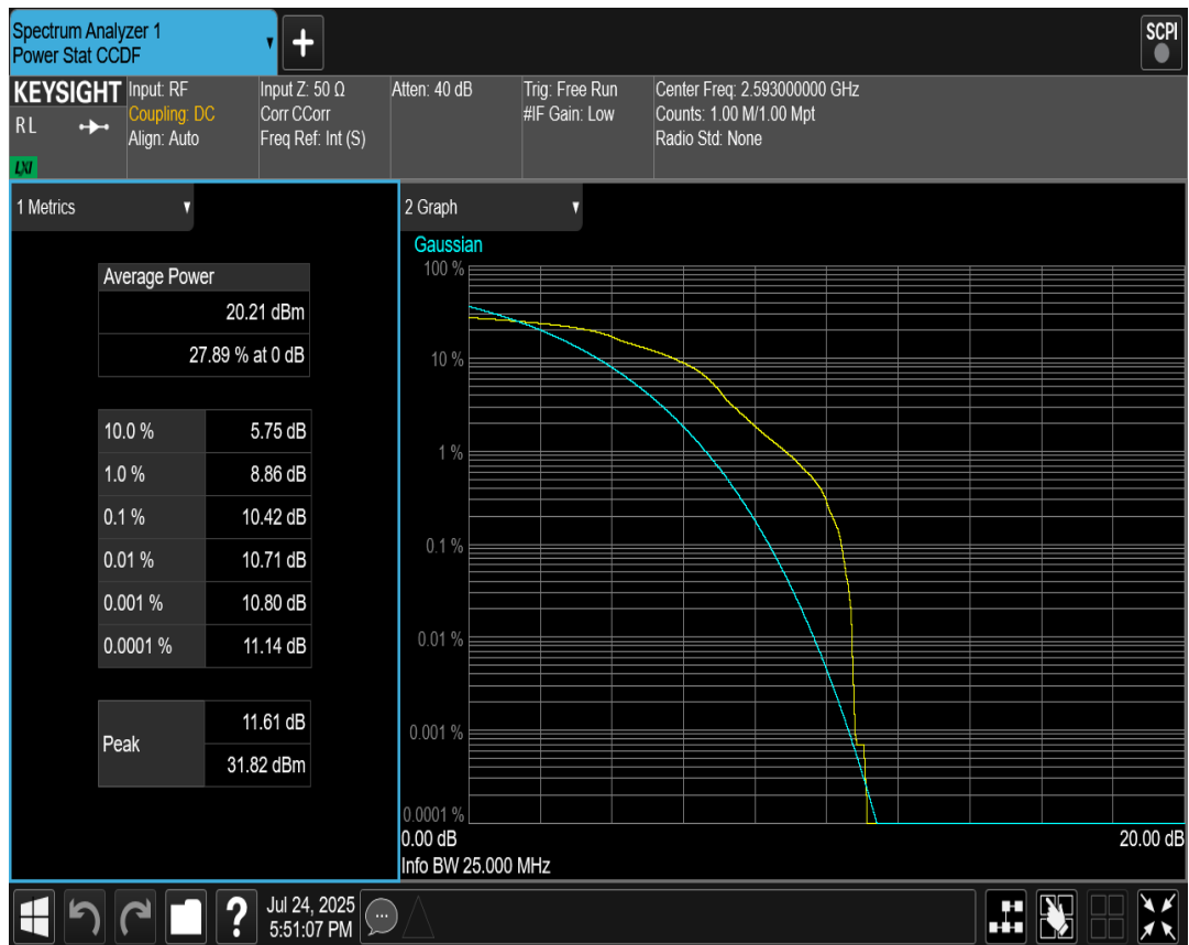
Band41 QPSK BW=10MHz Channel=40620 RB Size=1 Position=#0
