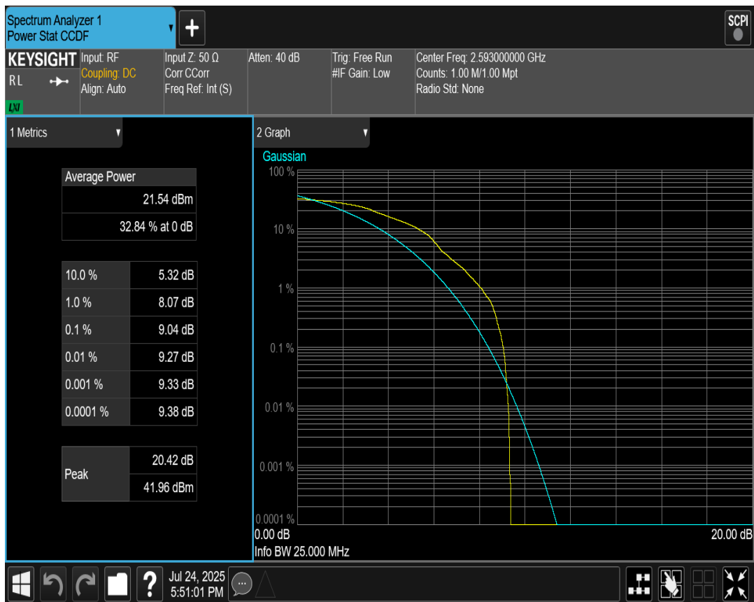
Band41 QPSK BW=5MHz Channel=40620 RB Size=1 Position=#0
