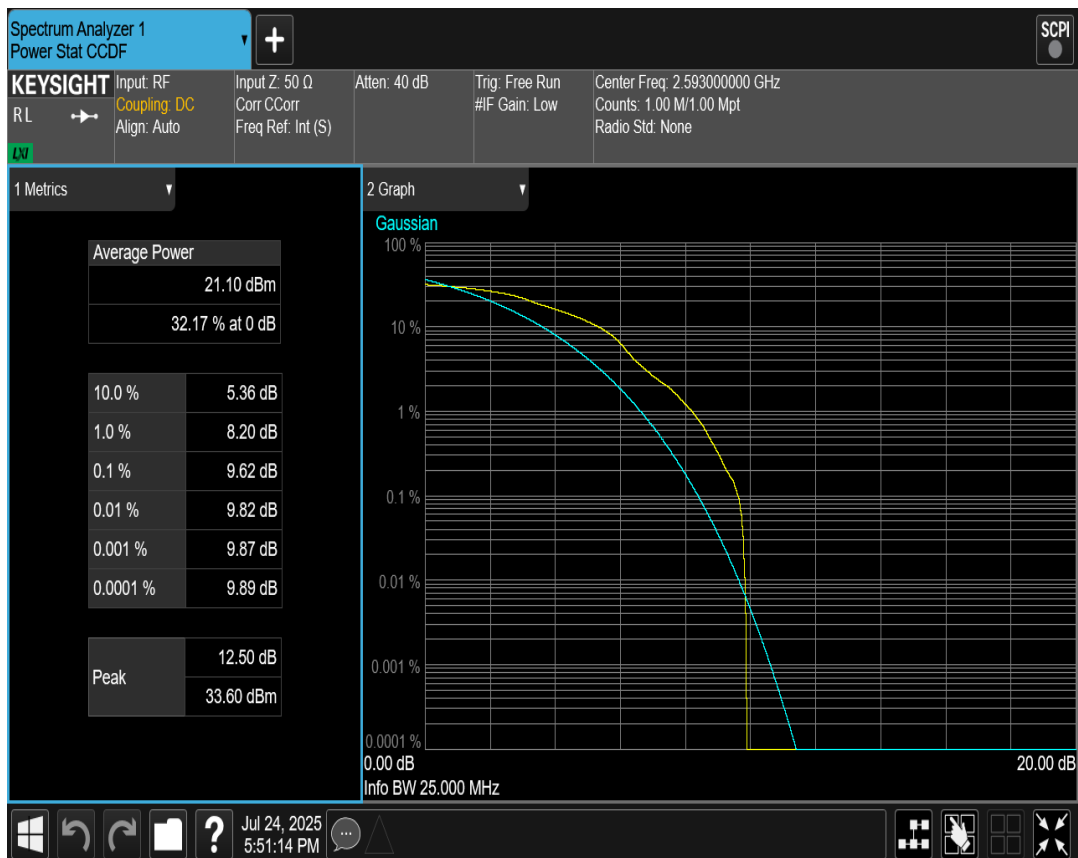
Band41 QAM16 BW=20MHz Channel=40620 RB Size=1 Position=#0
