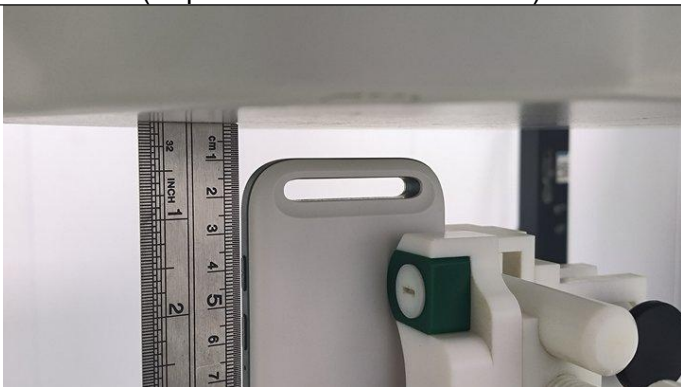
Top Side (Separation distance of 10mm)
