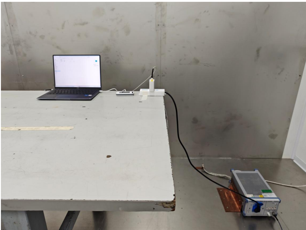
AC Conducted Measurement Photos
