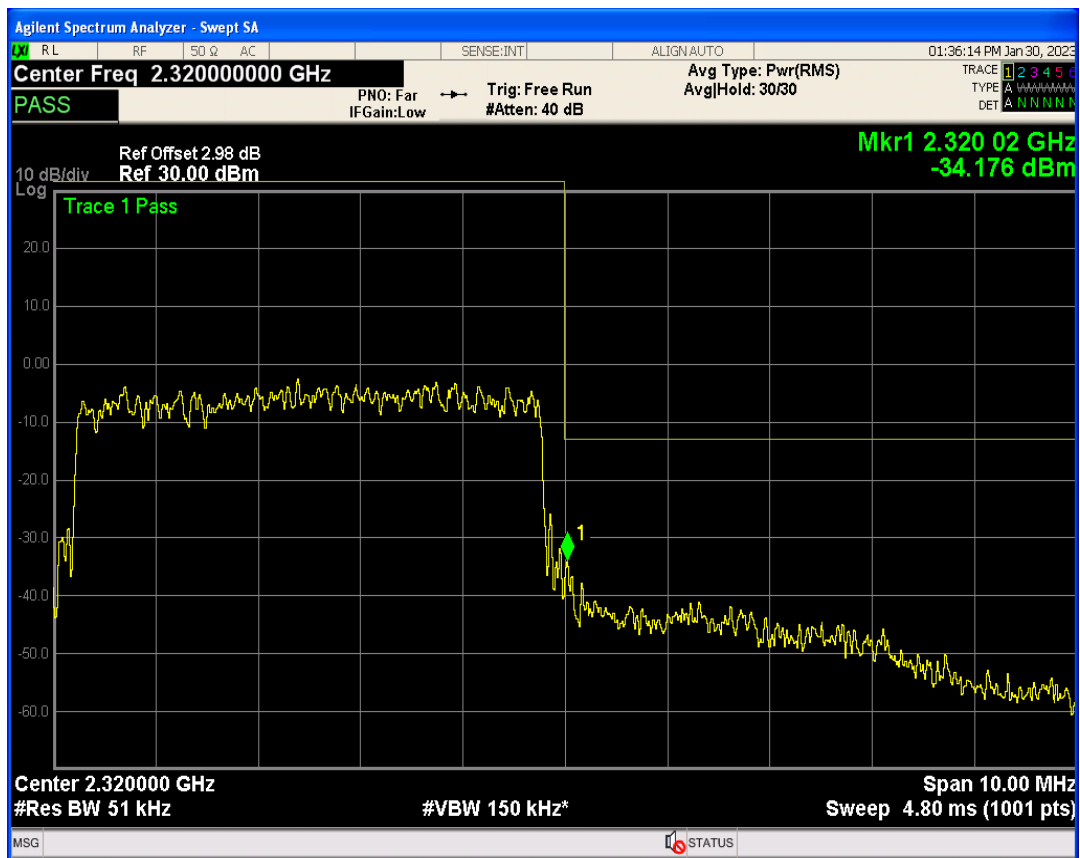
LTE Band40 QPSK BW=10MHz Channel=38750 RB Size=1 Position=#Max
