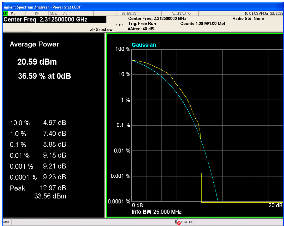
Band40 QAM16 BW=10MHz Channel=38775 RB Size=1 Position=#0
