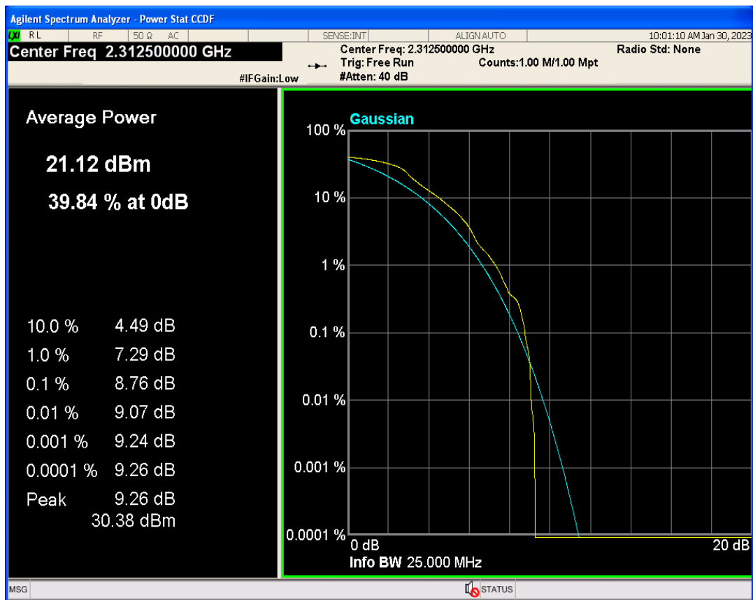
Band40 QAM16 BW=15MHz Channel=38775 RB Size=1 Position=#0
