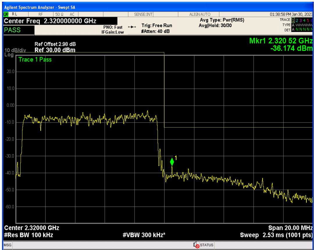
LTE Band40 QPSK BW=15MHz Channel=38775 RB Size=1 Position=#Max
