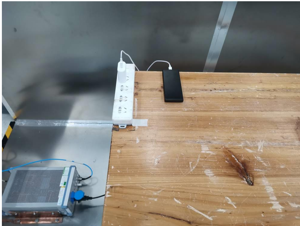
Photograph 3: Set-up photo for Conducted Emission
