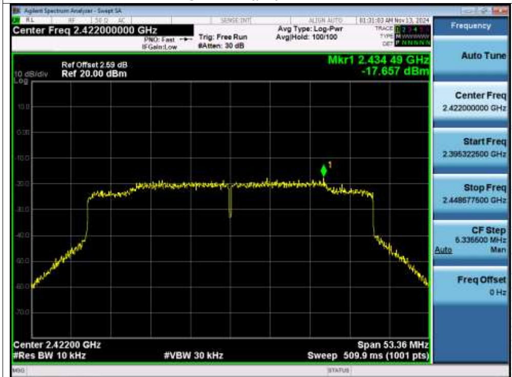
PSD NVNT ax40 2422MHz
