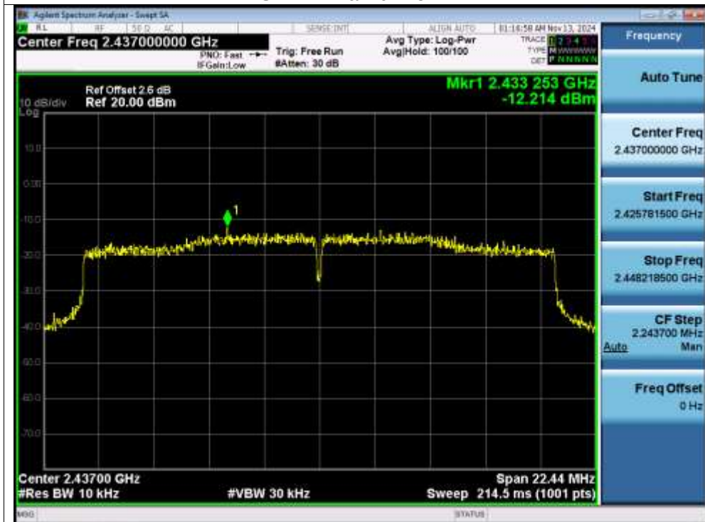
PSD NVNT ax20 2437MHz
