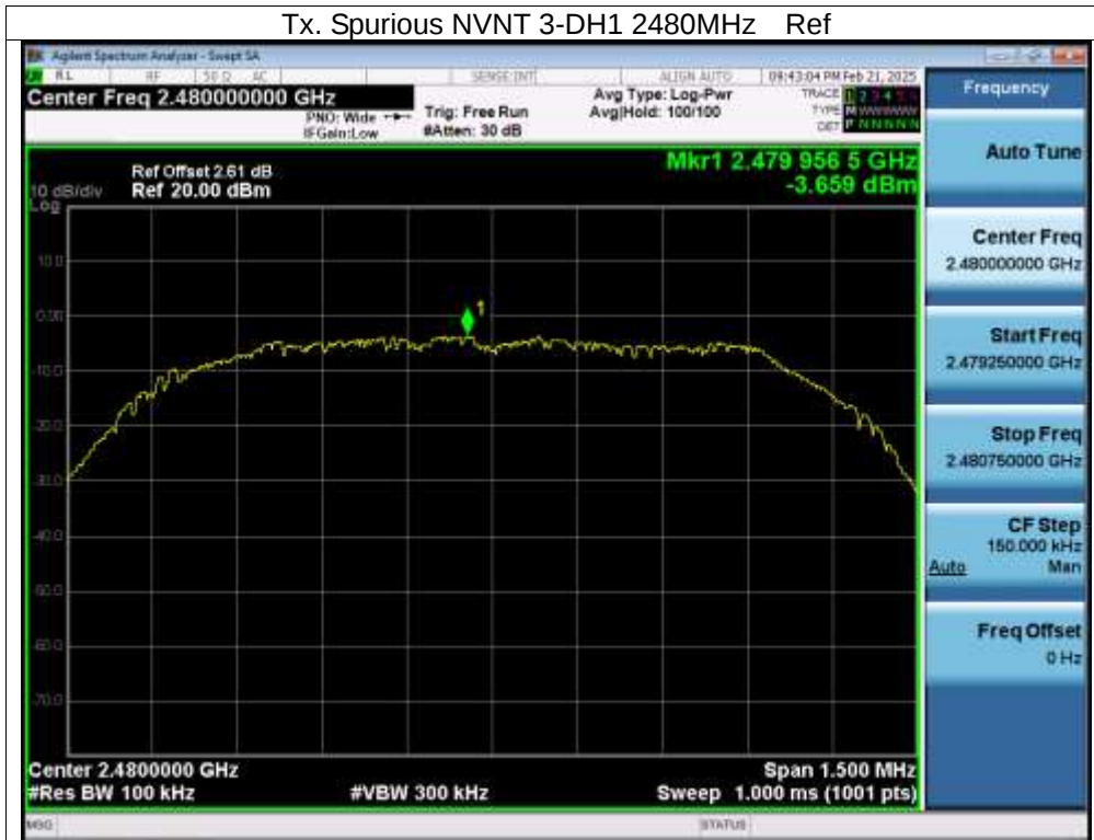
Tx. Spurious NVNT 3-DH1 2480MHz Emission
