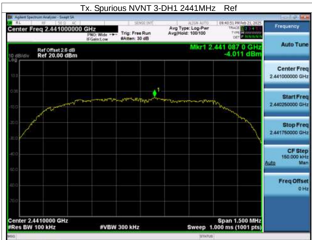
Tx. Spurious NVNT 3-DH1 2441MHz Emission
