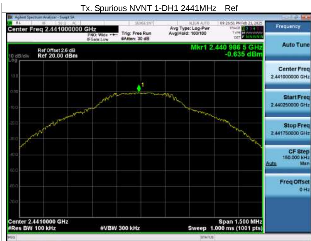
Tx. Spurious NVNT 1-DH1 2441MHz Emission
