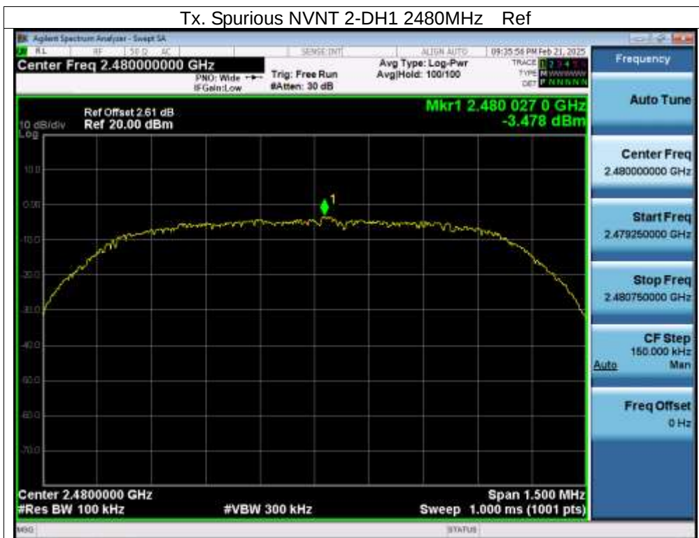
Tx. Spurious NVNT 2-DH1 2480MHz Emission
