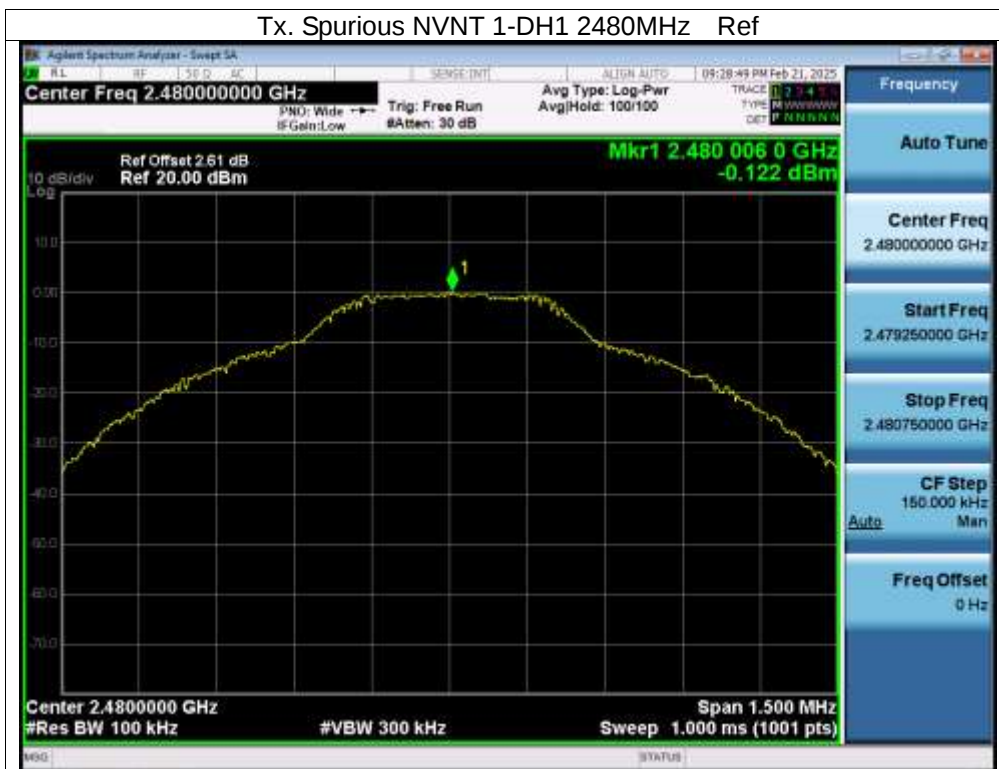
Tx. Spurious NVNT 1-DH1 2480MHz Emission
