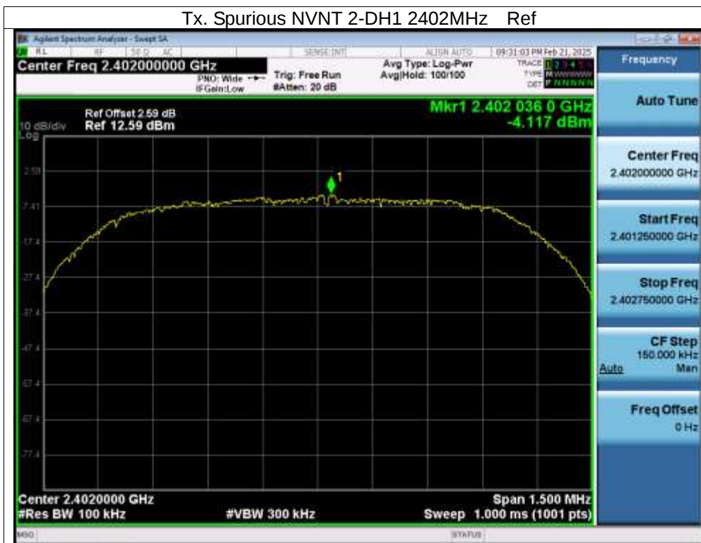
Tx. Spurious NVNT 2-DH1 2402MHz Emission
