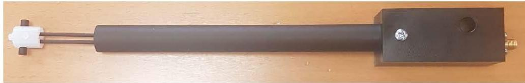
**Figure 1 – MVG COMOSAR Validation Dipole**
