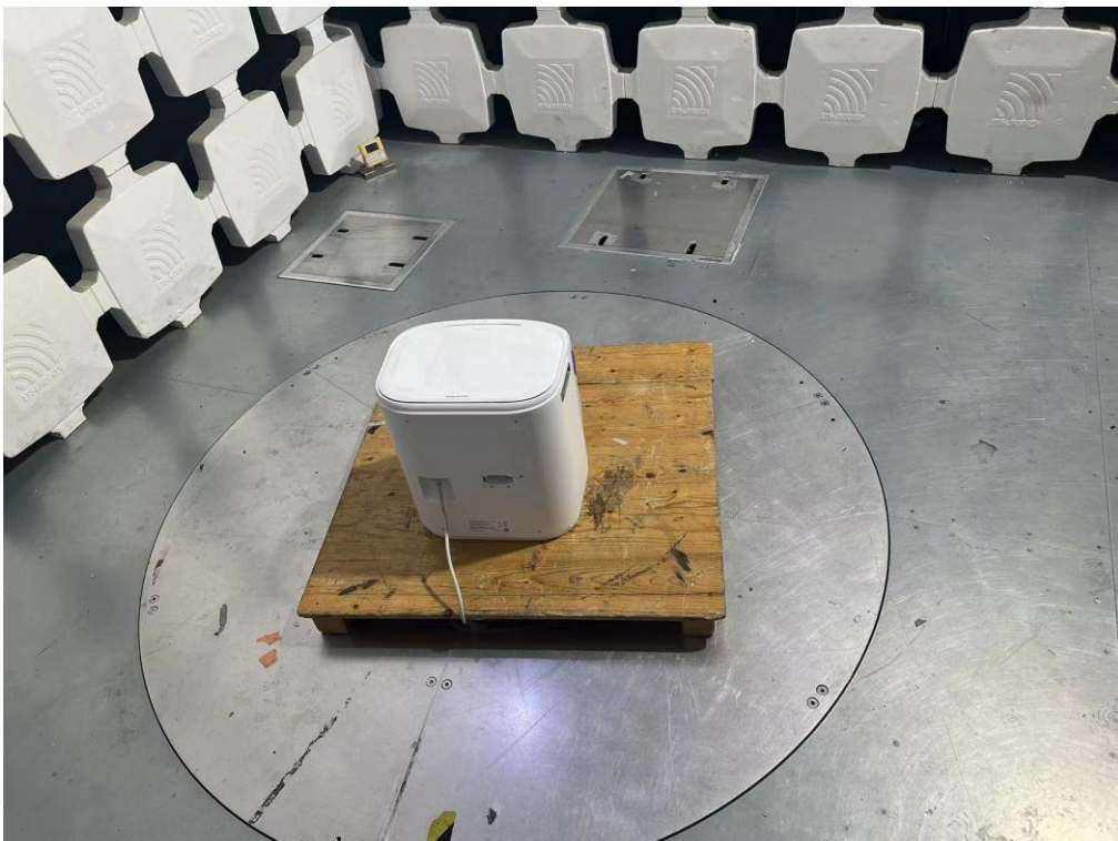
Above 1GHz (The EUT was placed in the center of the turntable)
