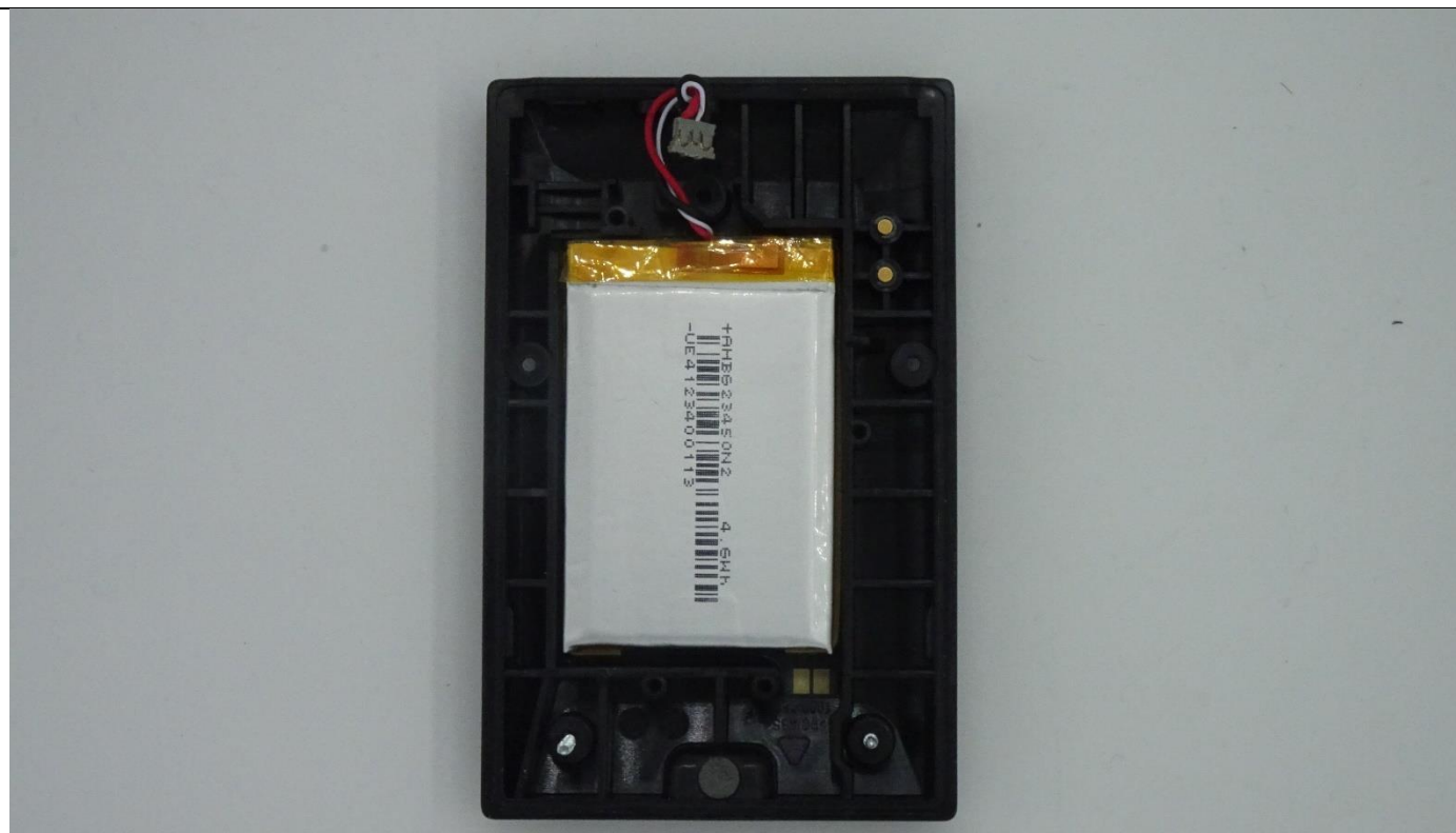
Picture 6, EUT, bottom cover inside with battery
