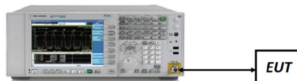
Figure 7-1. Test Instrument & Measurement Setup
