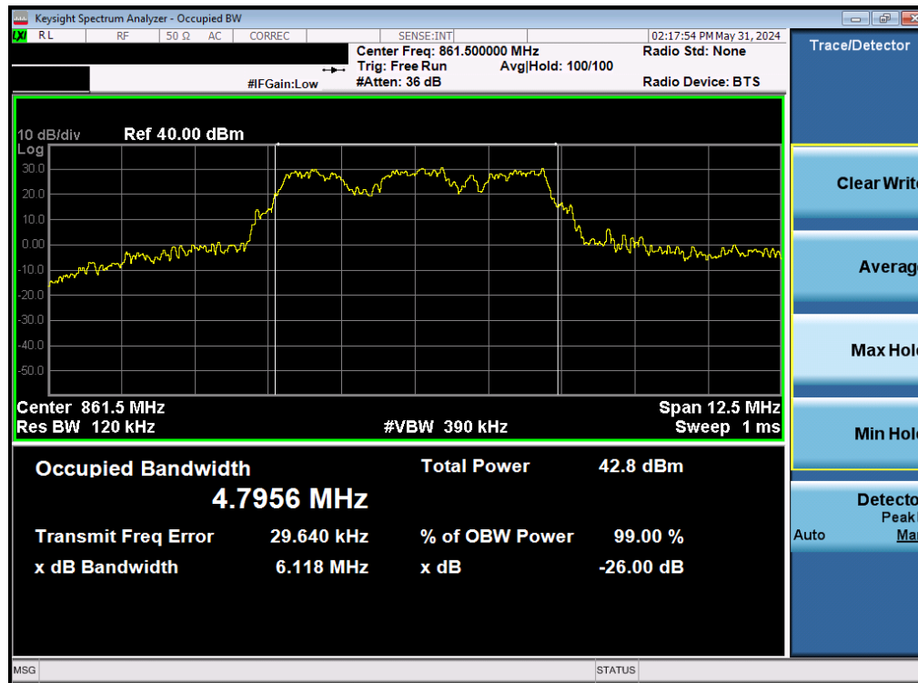
Plot 7-3. Occupied Bandwidth Plot (LTE Band 26)
