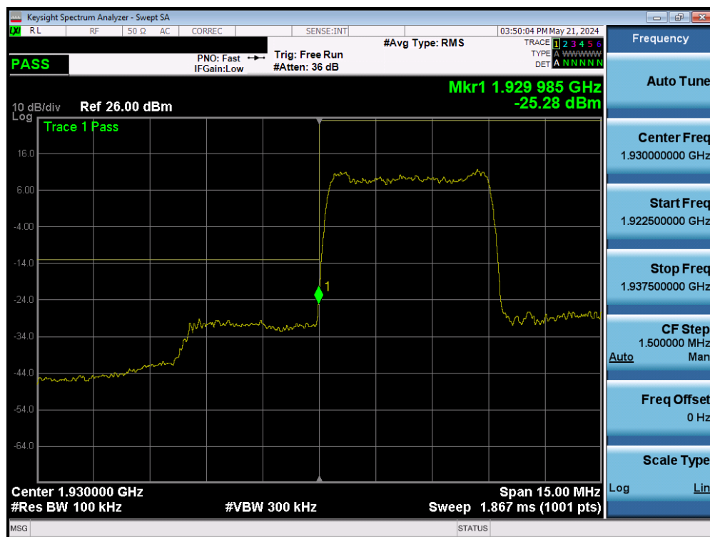
Plot 7-44. Lower Band Edge Plot (WCDMA PCS – Low Channel)
