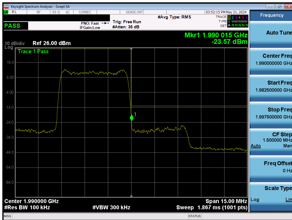
Plot 7-45. Upper Band Edge Plot (WCDMA PCS – High Channel)
