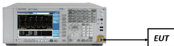
Figure 7-1. Test Instrument & Measurement Setup
