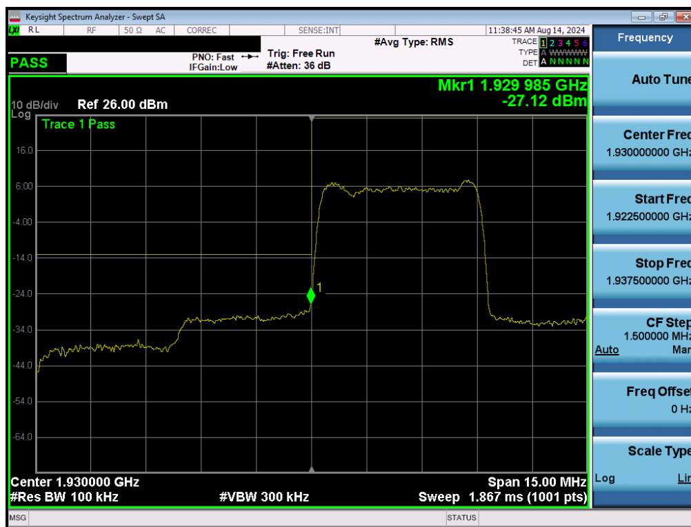
Plot 7-29. Lower Band Edge Plot (UMTS PCS – Ch. 9662)
