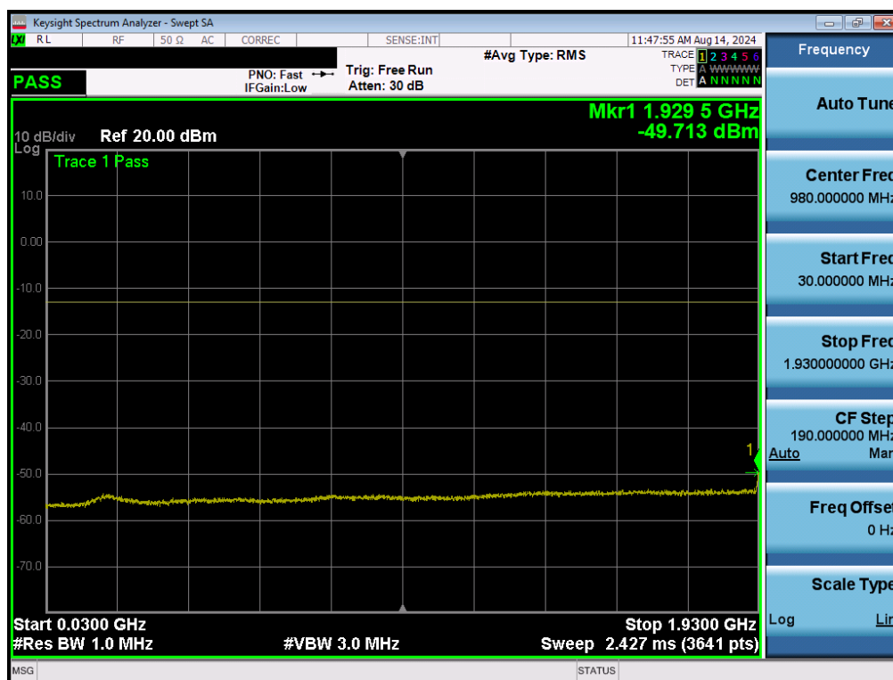
Plot 7-24. Conducted Spurious Plot (UMTS Ch. 9938)
