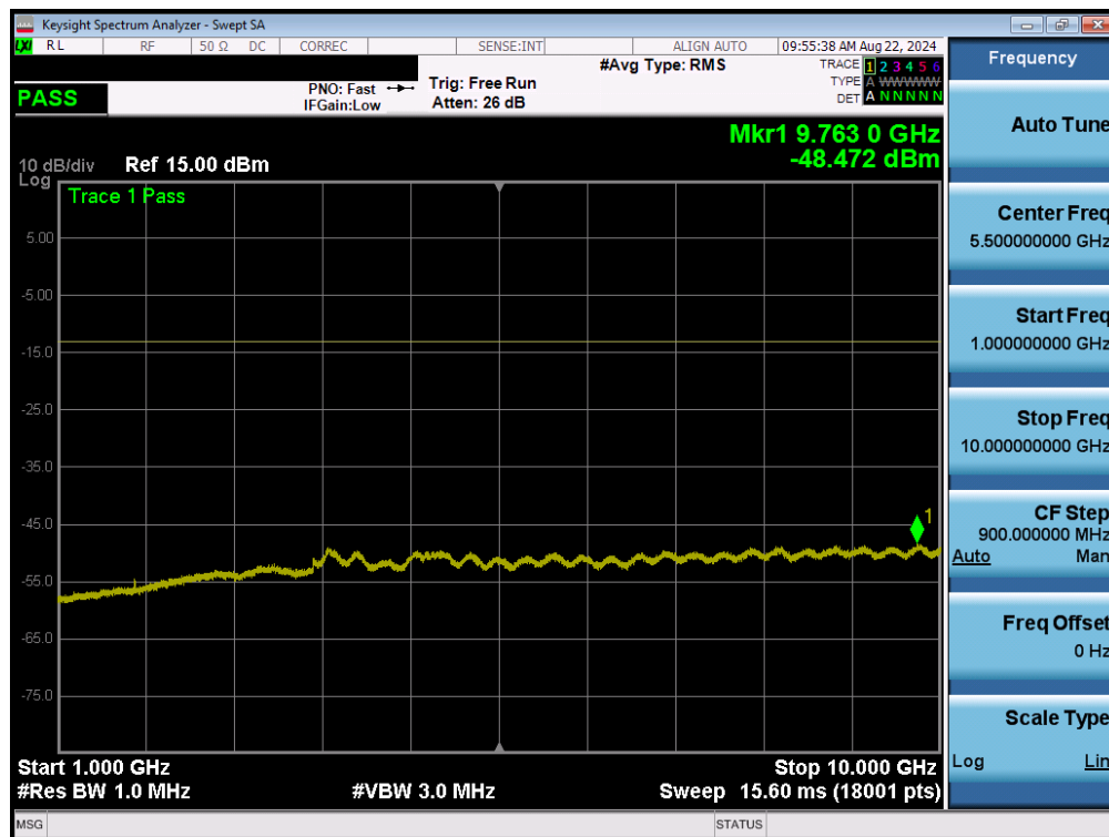
Plot 7-9. Conducted Spurious Plot – High Channel (UMTS Band 26 - 5MHz)
