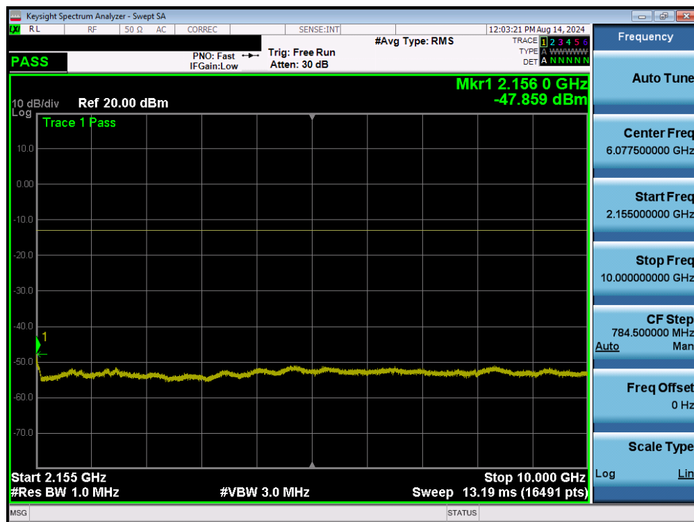
Plot 7-17. Conducted Spurious Plot (UMTS Ch. 1638- Mid Channel)
