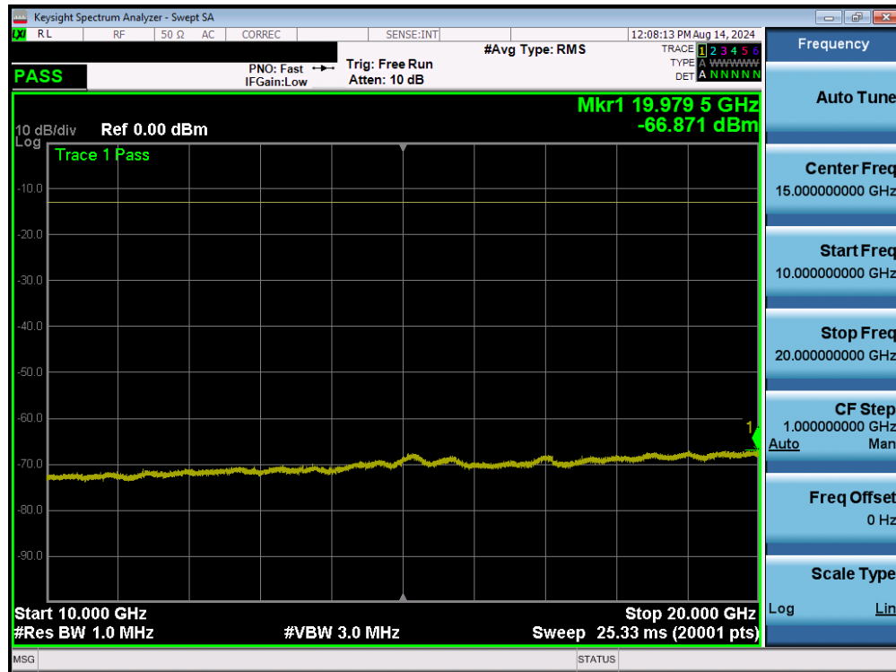
Plot 7-21. Conducted Spurious Plot (UMTS Ch. 1738- High Channel)
