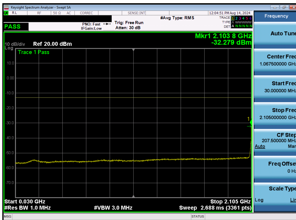
Plot 7-13. Conducted Spurious Plot (UMTS Ch. 1537- Low Channel)
