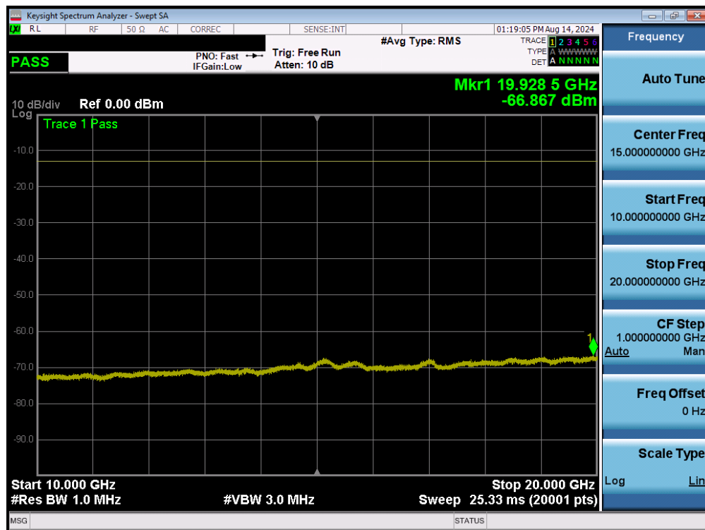
Plot 7-27. Conducted Spurious Plot (UMTS B12- Mid Channel)
