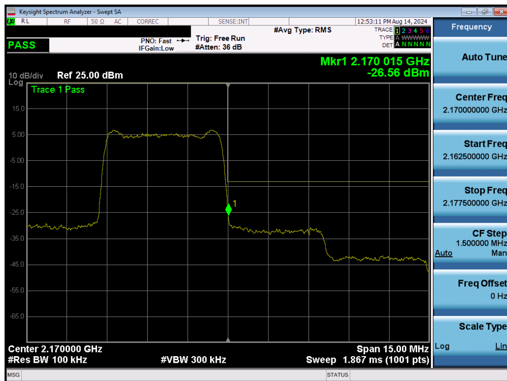
Plot 7-44. Upper Band Edge Plot (UMTS B10 – Ch. 1738)
