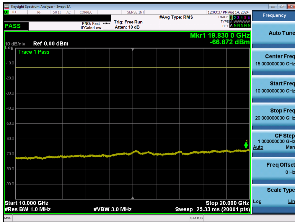
Plot 7-18. Conducted Spurious Plot (UMTS Ch. 1638- Mid Channel)
