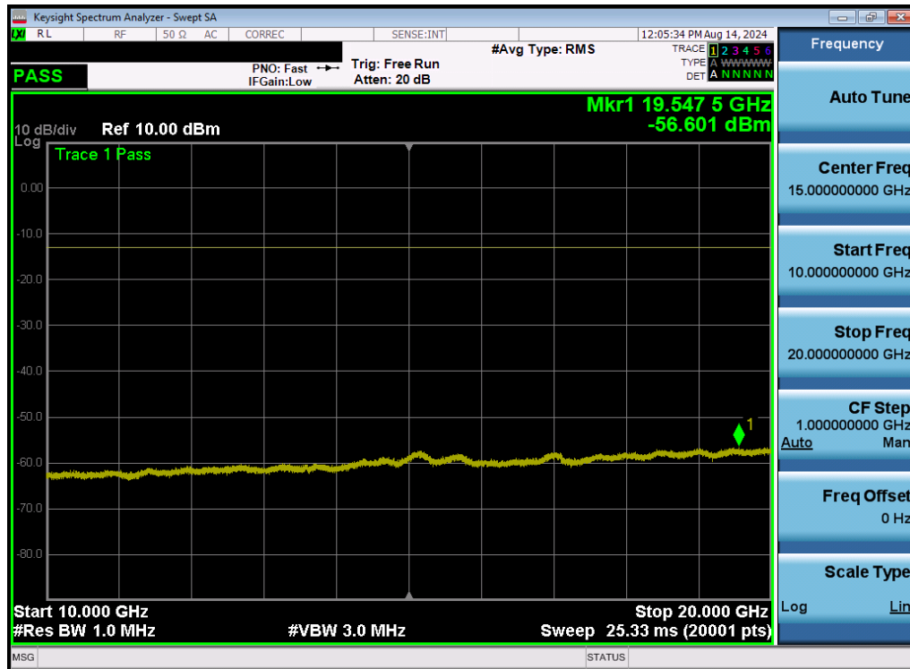
Plot 7-15. Conducted Spurious Plot (UMTS Ch. 1537- Low Channel)
