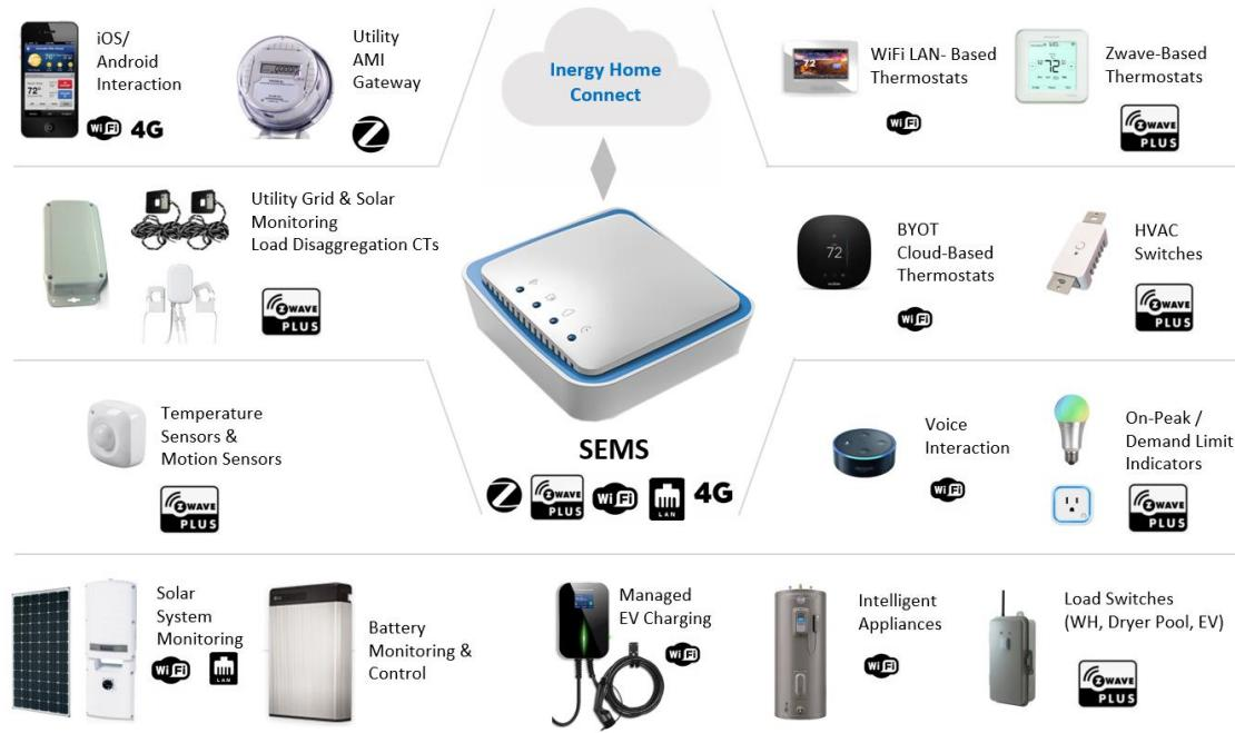
The SEMS connects to Inergy Home Connect (IHC) via Wi-Fi, LTE (optional) or Ethernet for real-time monitoring and control.
