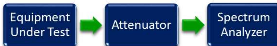
Figure 2. Occupied Bandwidth Test Setup
