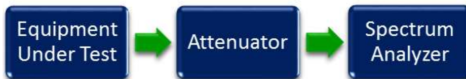
Figure 4. Conducted Spurious Emissions Test Setup
