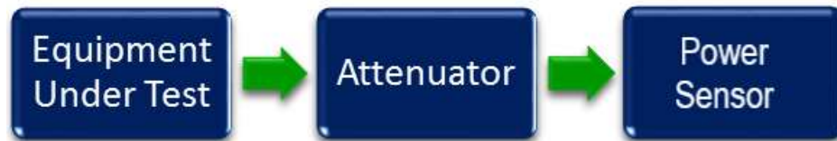
Figure 3. RF Power Test Setup
